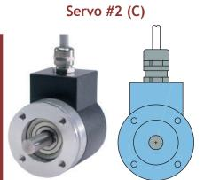
SERVO MOUNT #2 10-32 UNF-2B 6.35mm DEEP 4 x 90° on a 41,27mm PCD
