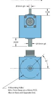
All dimensions are in mm with a tolerance of ±0.127mm or ±0.254 unless otherwise specified
