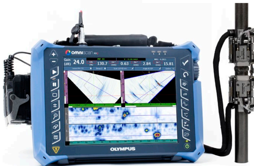
The COBRA scanner on a 0.84 in. pipe with two A15 PA probes with an OmniScan MX2 16:64 displaying two PA groups with sectorial scans and C-scans.
