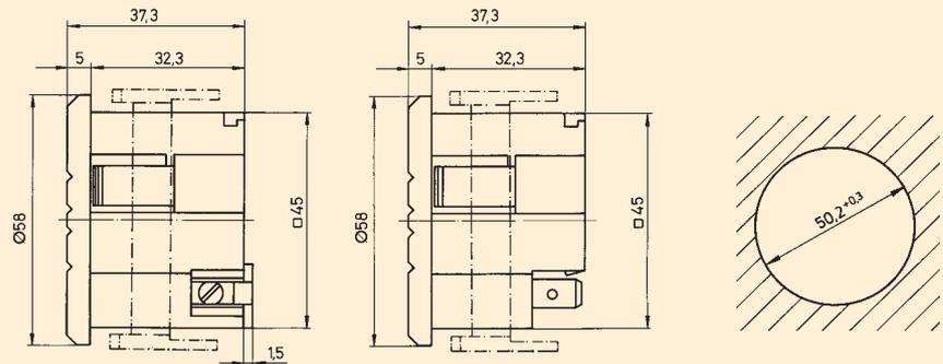
Front frame 48 x 48 mm, surface or DIN rail 35 mm (DIN 46277)
