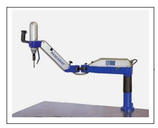
The machine is formed by a tilting arm being by means of a pneumatic spring, said arm being fitted through an intermediary union to a radial arm being revolvable around 360°.
