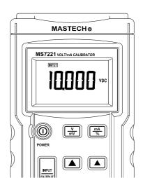
$\ensuremath{ \mbox{3Press}}$  the V mV conversion key  $\ensuremath{ 6}$ , make it indicate VDC
