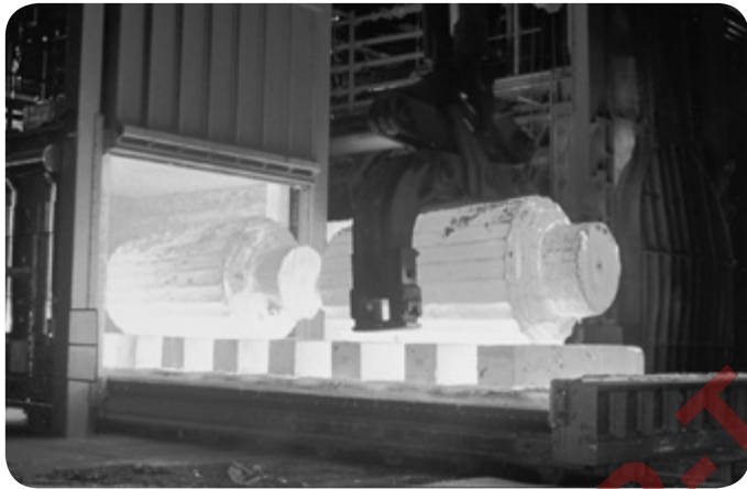
Metallurgical industry: forging furnace
