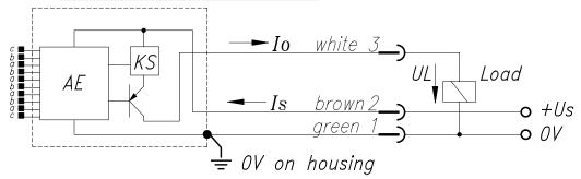
AE= detector electronics KS= short circuit protection
