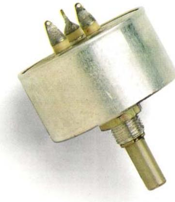
High quality container sealed, wirewound panel control of robust and reliable construction, with spindle and panel seals. Aluminium case and bushing; Anodized aluminium alloy spindle and fixing nut; nickel plated brass lid; silver plated brass tags insulated from lid by ceramic standoffs.
