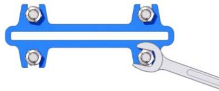
If the glandfollower nuts are pulled to hard, the force needed to operate the valve will increase, the valve function will be affected and the box packing lifetime will be shortened.
