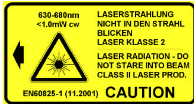
Fig. 3.2 Laser warning label affixed to the pyrometer
