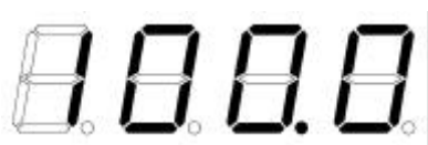
fig. 4: Emissivity ratio = 100.0 % for two-colour measurements
