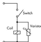
Effect of protective circuit at breaking
