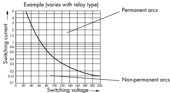
The area below the curve ensures a service life of  $\geq 1 \times 10^6$  operating cycles (90 % success of test samples).
