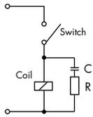
Effect of protective circuit at breaking
