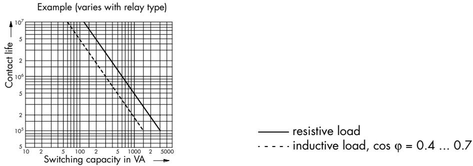
**Parameters for finding the AC correct switching capacity curve**
