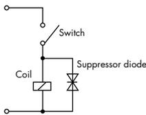
Effect of protective circuit at breaking
