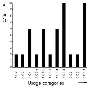
Ic = making-, breaking current
