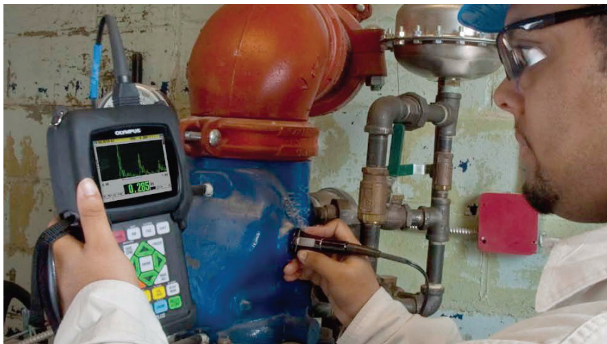
Figure 1-1 Measuring thicknesses with the 38DL PLUS
