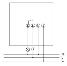
The device can be manually activated with a circuit breaker. After releasing the button (return of power) the device switches on (for at least 40 secs or for the time set on the device).
