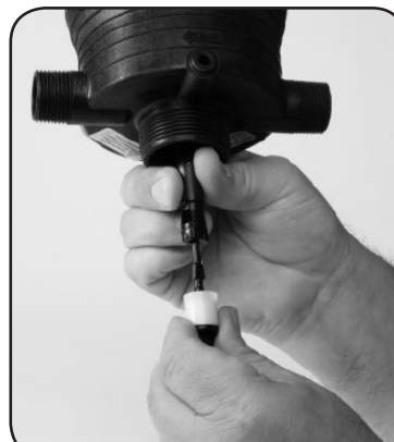
Step 8. Reinstall lower shaft with new dosage piston by turning 90° to lock in place.
