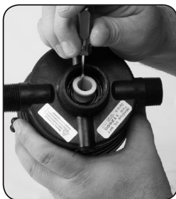
Step 4. Remove #82 SHAFT SEAL SPACER.
