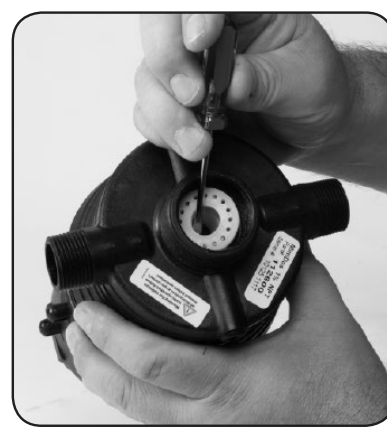
Step 3. Remove #16 Gasket.
