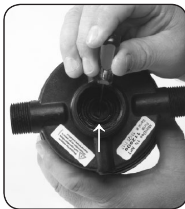
Step 5. Remove #17 O-ring and replace.
