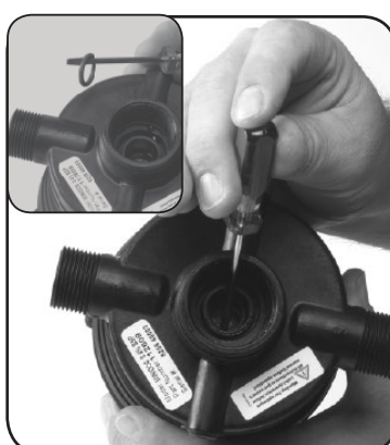
Step 5. Remove #17 O-ring.
