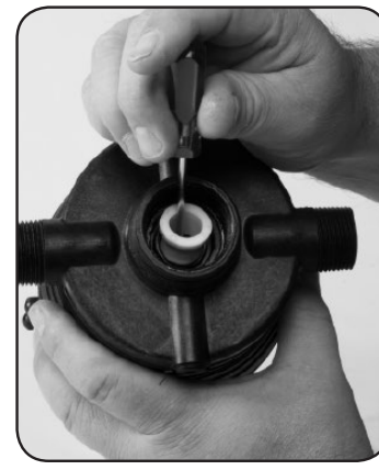
Step 3. Remove #83 SHAFT SEAL SPACER.
