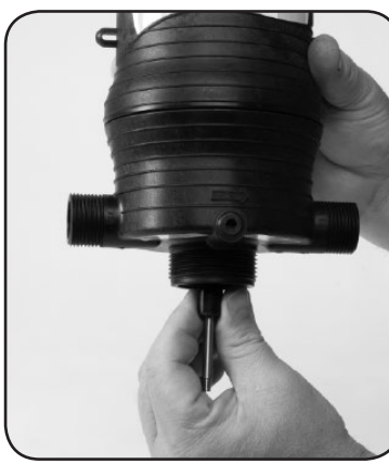
Step 8. Replace #51 SHAFT ASSEMBLY.
