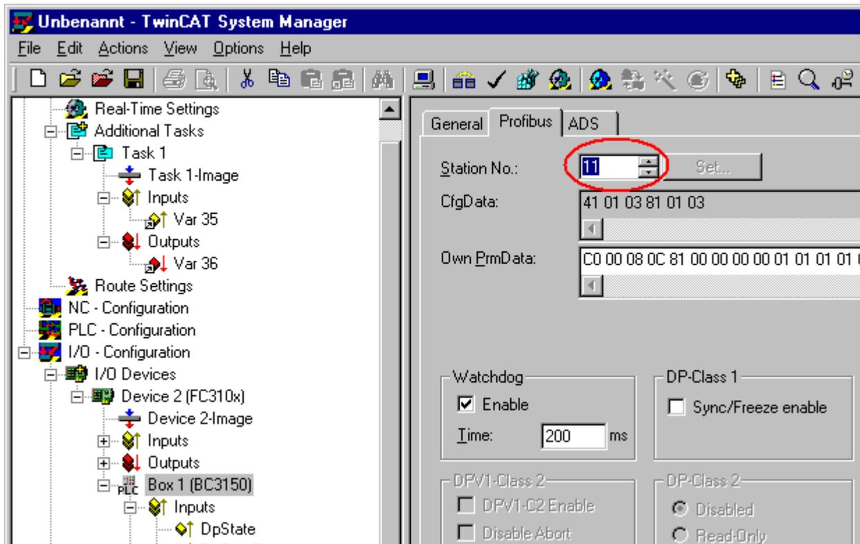
Activate the configuration and start the system. The TwinCAT icon (bottom right on the desktop) should be green. The bus LED on the BC3150 should also be green. Should this not be the case, check the BC3150 address and the physical connection to the PROFIBUS master (terminal resistances etc.).
