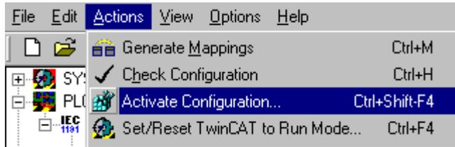
The current configuration is uploaded to the BX. The display will show *Store Config*, and the BUS and I/O LED will flash. After the configuration has been transferred successfully to the BX, the BX display should show *TwinCAT Config*. The required program can now be transferred to the BX (program download via the fieldbus).
