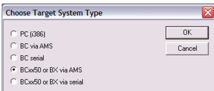
After your program has been created, select the target system under the *Online* toolbar. TwinCAT must be running to do this. In the example, this is the Ethernet card with Box 1 and the Runtime 1 of the Bus Terminal Controller.
