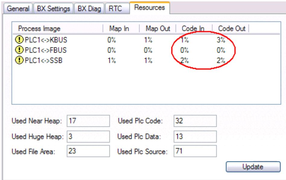
Fig. 1: Memory for code mapping
