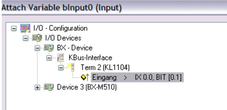
In the TwinCAT configuration, all Bus Terminals have fixed addresses. If a Bus Terminal is inserted, the whole address range may be shifted. Many data are unnecessary and take up valuable address memory space. The TwinCAT configuration rectifies this disadvantage. Allocated variables can be linked freely with a Bus Terminal. Parameterization is carried out in the System Manager, and the configuration is then transferred to the BX (see TwinCAT configuration).
