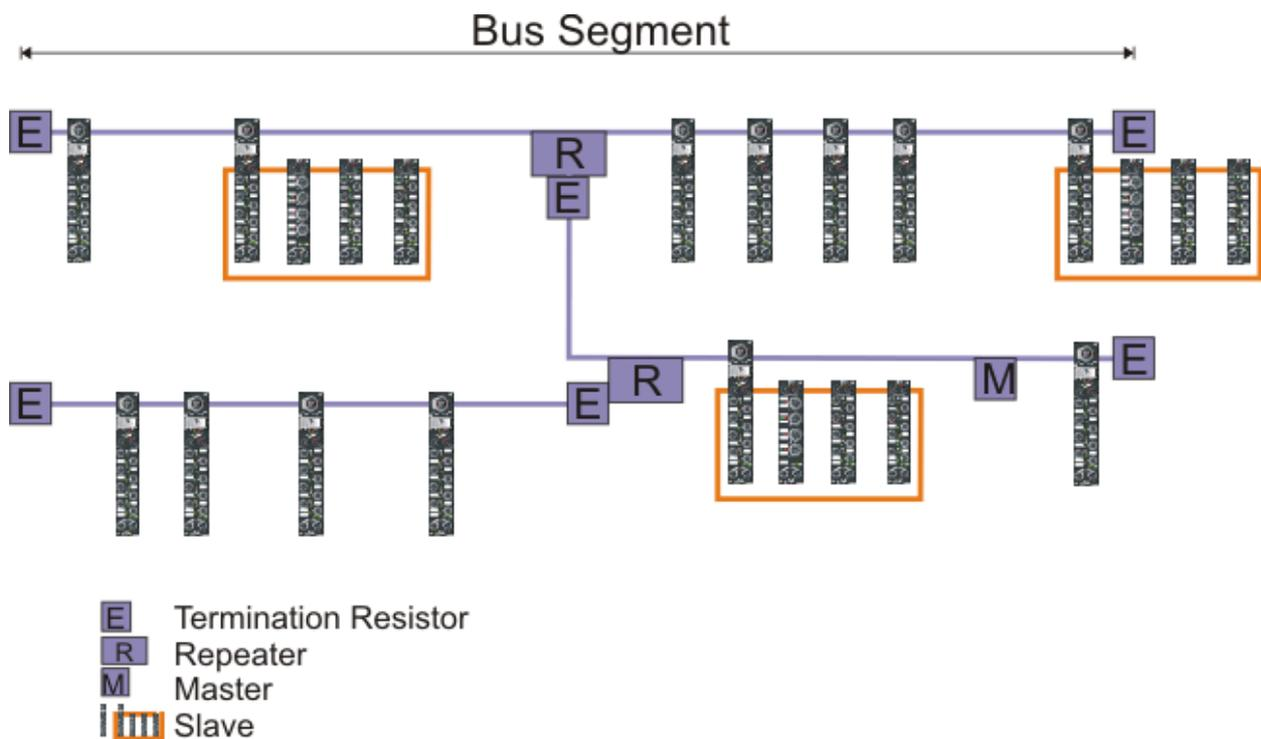
Fig. 1: RS485 topology with 3 segments and 2 repeaters.
