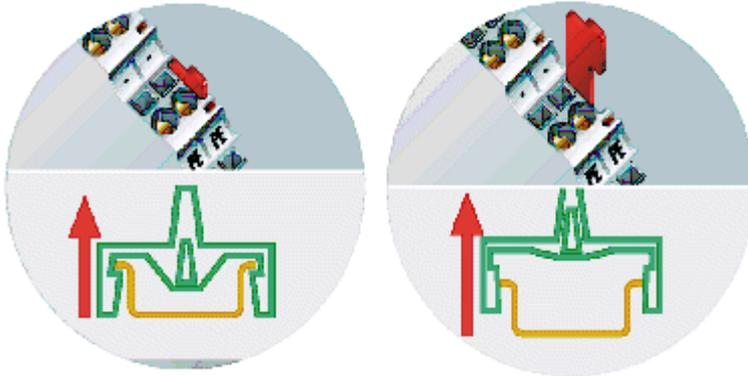
Up to 64 Bus Terminals can be attached to the Bus Coupler on the right hand side. When plugging the components together, be sure to assemble the housings with groove and tongue against each other. A properly working connection can not be made by pushing the housings together on the mounting rail. When correctly assembled, no significant gap can be seen between the attached housings.
