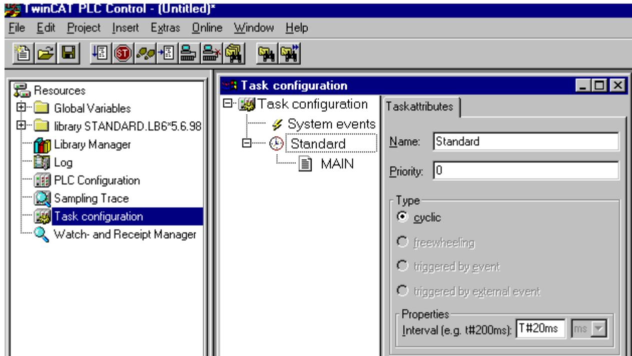
In the default setting, the PLC program is called every 20 ms, as long as the general cycle time is less than 20 ms. The cycle time can be measured in the System Manager in order to determine your system load. To ensure trouble-free operation, the set task time should be 20 to 30 % higher than the measured cycle time. A precise cycle time breakdown can be found under K-Bus tab description.
