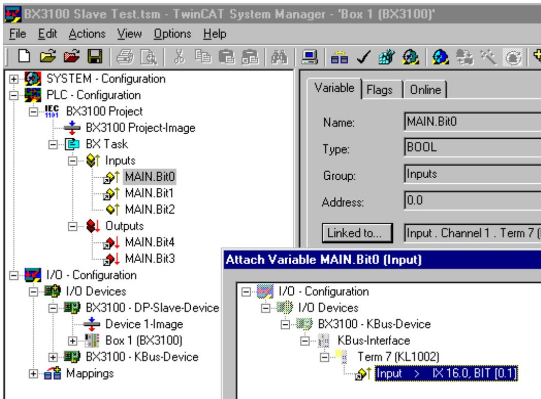
Once all links have been created, activate the configuration *Actions/Activate Configuration* (Ctrl+Shift+F4) and start TwinCAT *Set/Reset TwinCAT to Run Mode*. Ensure that the correct target system is selected (bottom right in the System Manager window).
