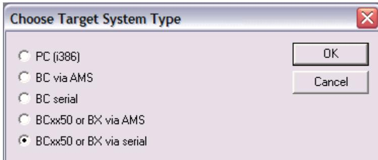
The settings for the serial interface, port number, baud rate etc. are found under Online/Communication parameters in PLC Control.
