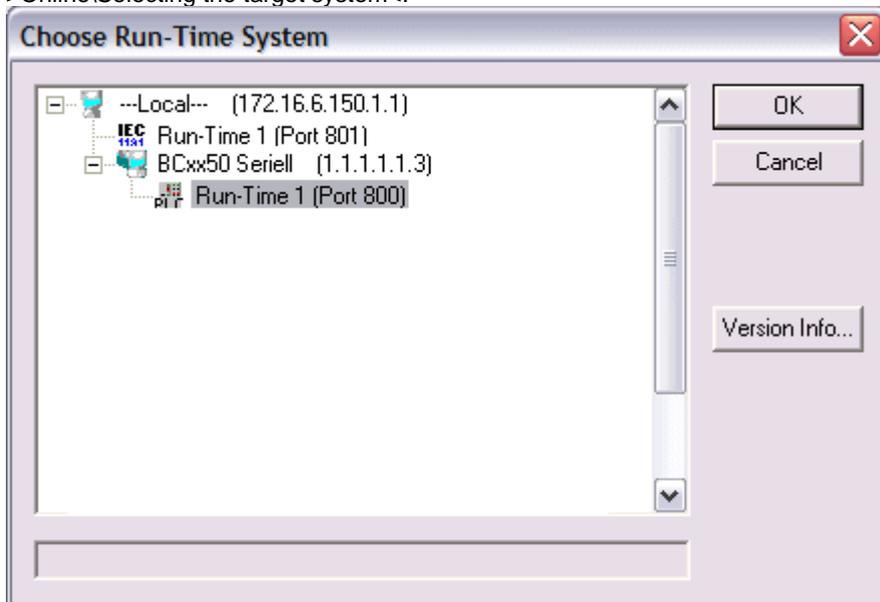
Load the project into the controller (>Online>Login<) and Start the program (>Online\Start<). The PLC LED on the BC3150 should now be orange.
