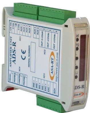
ADS-R is a digital measuring amplifier for strain gauges bridge, including a 24 bit acquisition circuit with programmable gain and 3 analog outputs towards a supervision unit.
