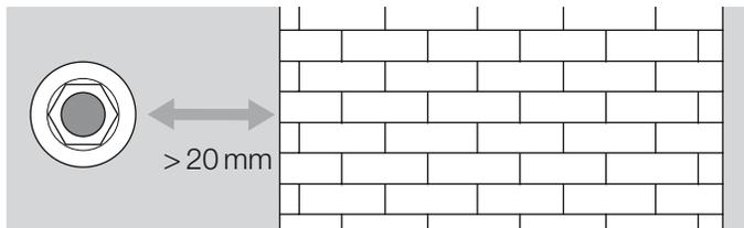
The GRS/GRSF must not be in contact with masonry. Minimum clearance 20 mm (0.8 inch).
