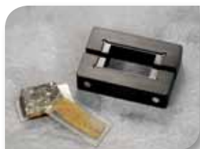
Petrographic glass slide hand-held holder for 27 x 46mm glass slides
