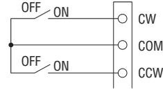
● Use a small-capacity contact type relay capable of opening and closing 14 VDC, 10 mA.
