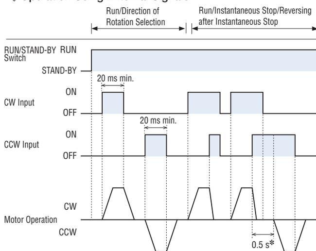
\* Motor does not run for 0.5 s after instantaneous stop, if a reversing run signal is input.
