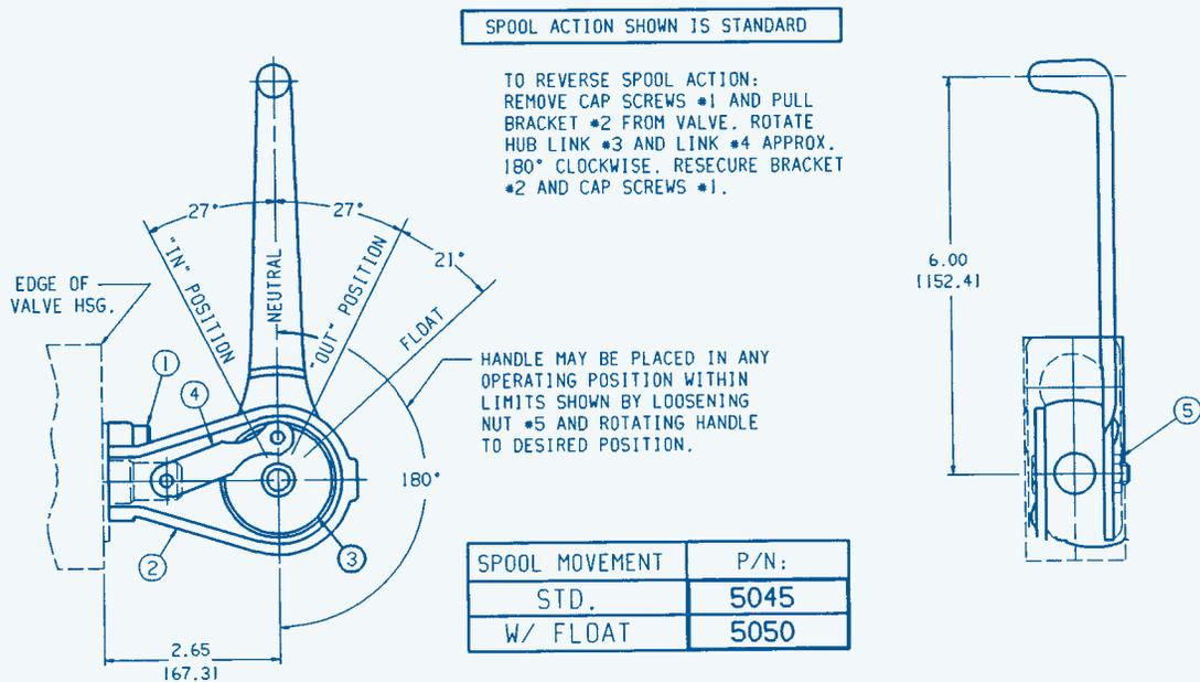
FOR PARALLEL AND CONVENTIONAL CIRCUIT SECTIONS
