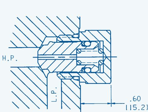
THE ANTI-CAVITATION CHECK VALVE OPENS WHEN L.P. PASSAGE PRESSURE EXCEEDS THE H.P. PASSAGE PRESSURE.
