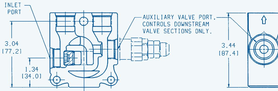
MID-INLET SECTIONS ARE USED IN-BETWEEN SPOOL SECTIONS EITHER TO ADD FLOW TO THE DOWNSTREAM SPOOL SECTIONS "COMBINER" OR TO INTRODUCE A "SEPARATE FLOW" CONDITION TO THE DOWNSTREAM SPOOL SECTIONS. MID-INLET SECTIONS ARE COUNTED AS A SPOOL SECTION WHEN DETERMINING TIE ROD KIT NUMBER.
