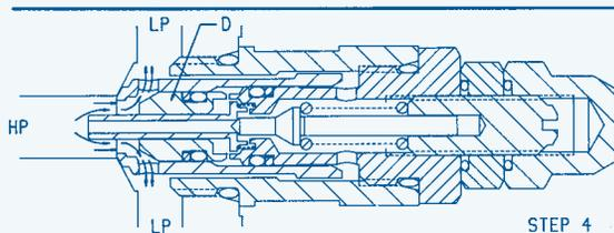
The imbalance of pressure on the inside as compared to that of the high pressure port "HP," forces the relief valve poppet "D" to open and relieve the oil directly to the low pressure chamber "LP" in the valve.
