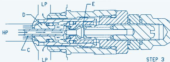
The loss of oil behind Poppet "C," effected by the opening of pilot poppet "E," causes poppet "C" to move back and seat against pilot poppet "E." This shuts off the oil flow to the area behind relief valve poppet "D," and causes a low pressure area internally.
