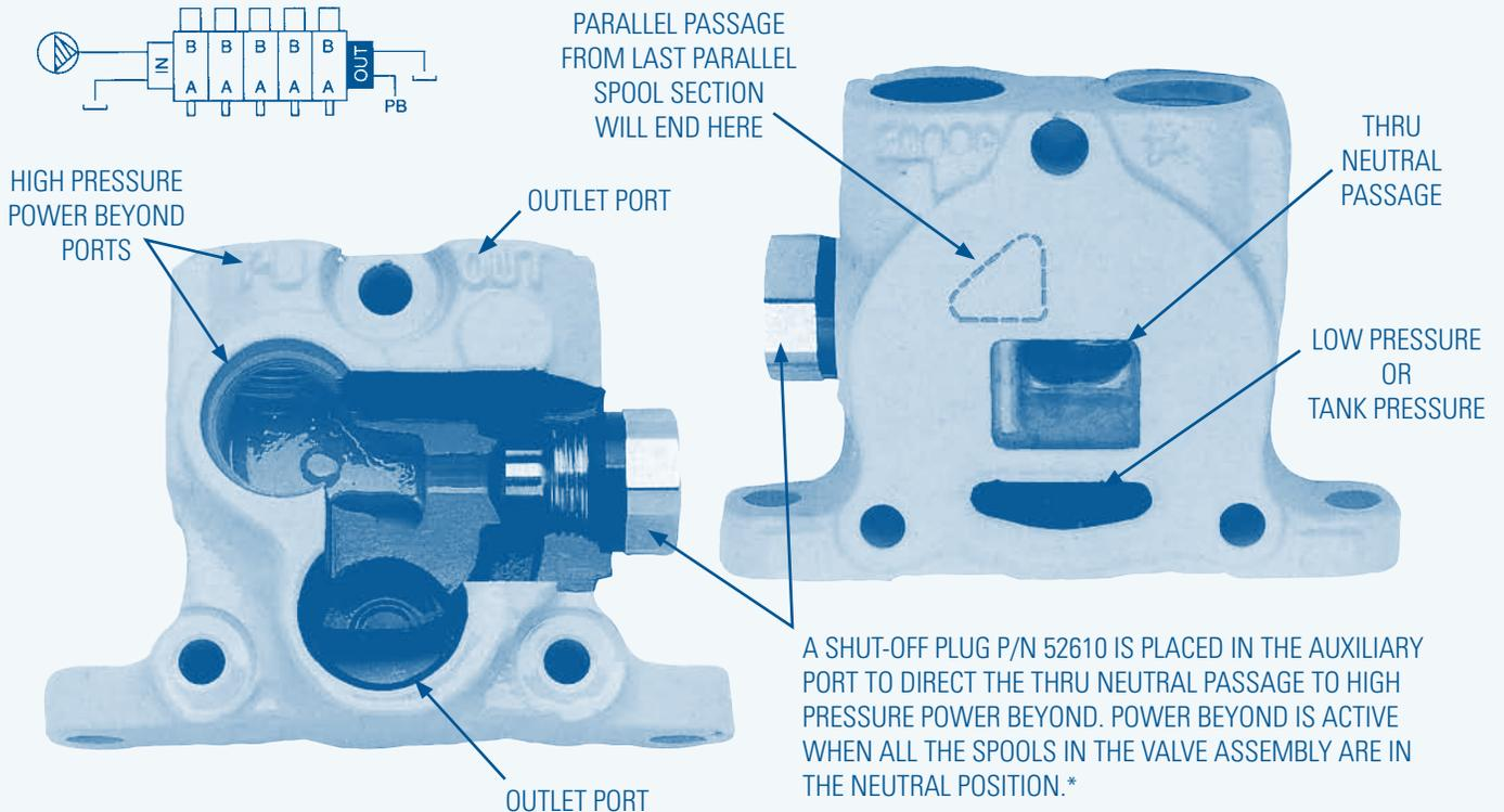
\*Exception: series circuit valve section assemblies return discharged oil to neutral passage. (See page 18 for other circuit options)
