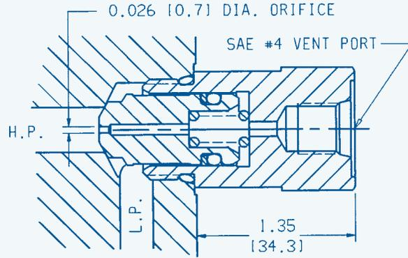
THE VENTABLE ANTI-CAVITATION CHECK VALVE OPENS WHEN THE L.P. PASSAGE PRESSURE EXCEEDS THE H.P. PASSAGE PRESSURE OR WHEN THE VENT PORT IS OPENED TO TANK.
