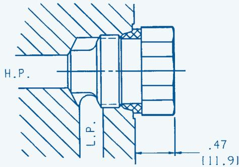
THE SHUT-OFF PLUG IS USED TO SHUT-OFF THE L.P. PASSAGE FROM THE H.P. PASSAGE IN ALL THE AUX. VALVE PORTS. IT IS USED TO PLUG THE AUX. VALVE PORT WHEN AN AUX. VALVE IS NOT REQUIRED. THE SHUT-OFF PLUG IS ALSO USED IN THE OUTLET SECTION TO ACTIVATE THE POWER BEYOND PORT(S).
