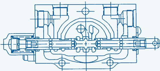
SERIES CIRCUITRY IS ACCOMPLISHED BY USING A HOLLOW SPOOL
