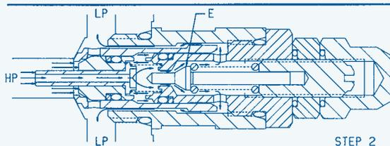
The oil pressure in the high pressure port "HP" has reached the setting of the pilot poppet spring force and unseats the pilot poppet "E." Oil flows around the poppet – through the cross drilled holes and to the low pressure area "LP."
