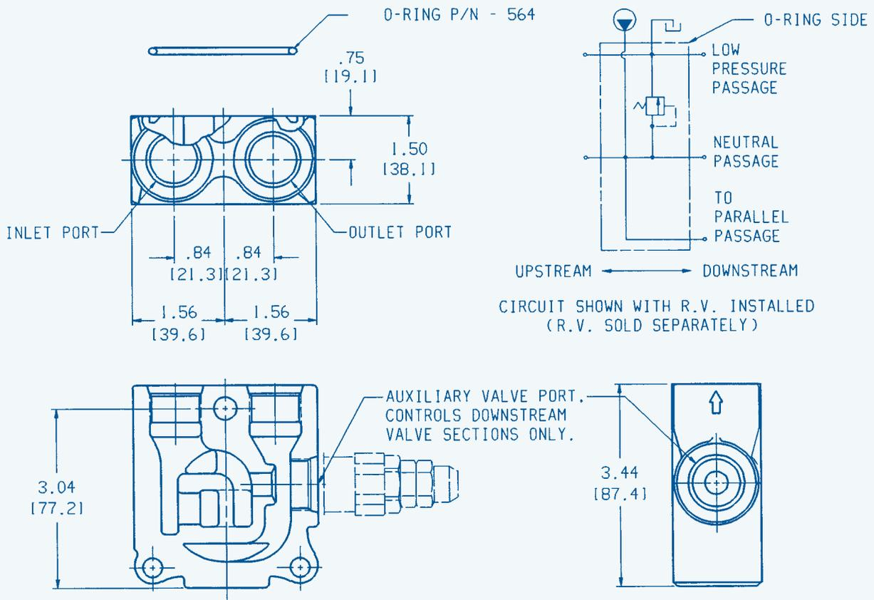
MID-INLET SECTIONS ARE USED IN-BETWEEN SPOOL SECTIONS EITHER TO ADD FLOW TO THE DOWNSTREAM SPOOL SECTIONS "COMBINER" OR TO INTRODUCE A "SEPARATE FLOW" CONDITION TO THE DOWNSTREAM SPOOL SECTIONS. MID-INLET SECTIONS ARE COUNTED AS A SPOOL SECTION WHEN DETERMINING TIE ROD KIT NUMBER.
