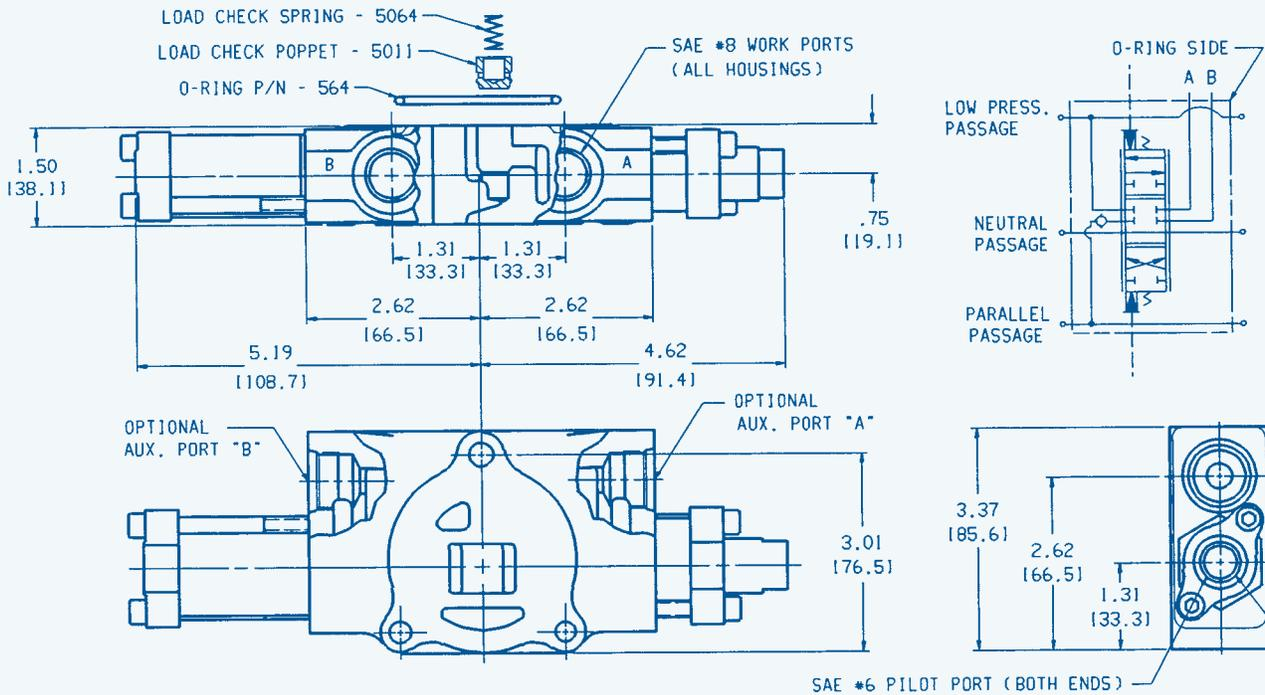
WHEN PILOT PRESSURE IS APPLIED TO THIS PILOT PORT SECTION SENSES HI-PRESS. "A", LOW PRESS. "B". WHEN PILOT PRESSURE IS APPLIED TO OPPOSITE PILOT PORT SECTION SENSES HI-PRESS. "B", LOW PRESS. "A". WHEN NO PILOT PRESSURE IS APPLIED SECTION SENSES NEUTRAL.
