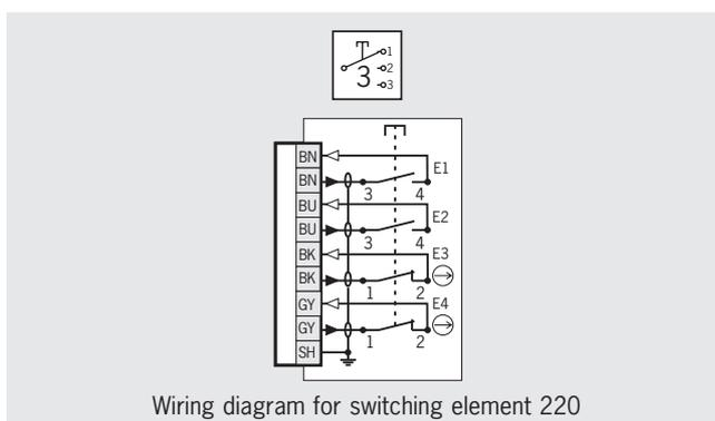
The normally open contact E1 and the positively driven contact E3 as well as the normally open contact E2 and the positively driven contact E4 can be connected externally in series. In this way a dual-channel design is achieved.
