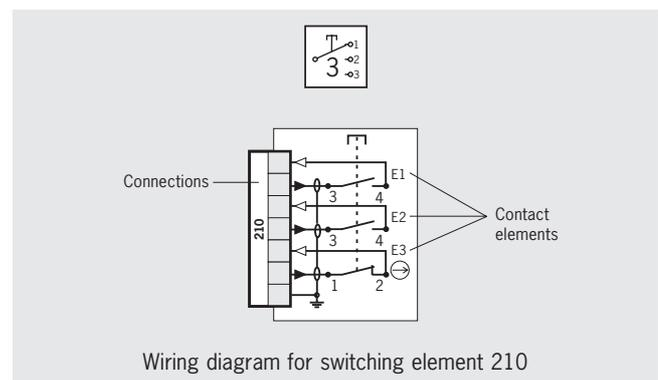
The wiring diagram shows the switching element in the free position (enabling switch not actuated).
