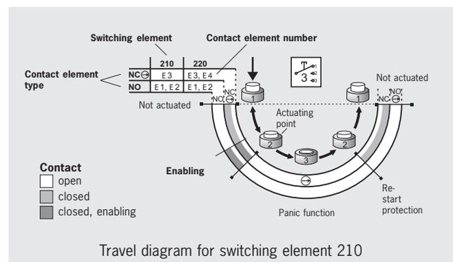
As in this example, in some cases several switching elements are combined in one travel diagram. Here, along with the switching element 210 with the contact elements E1, E2 and E3, there is also the switching element 220 with the contact elements E1 to E4.
