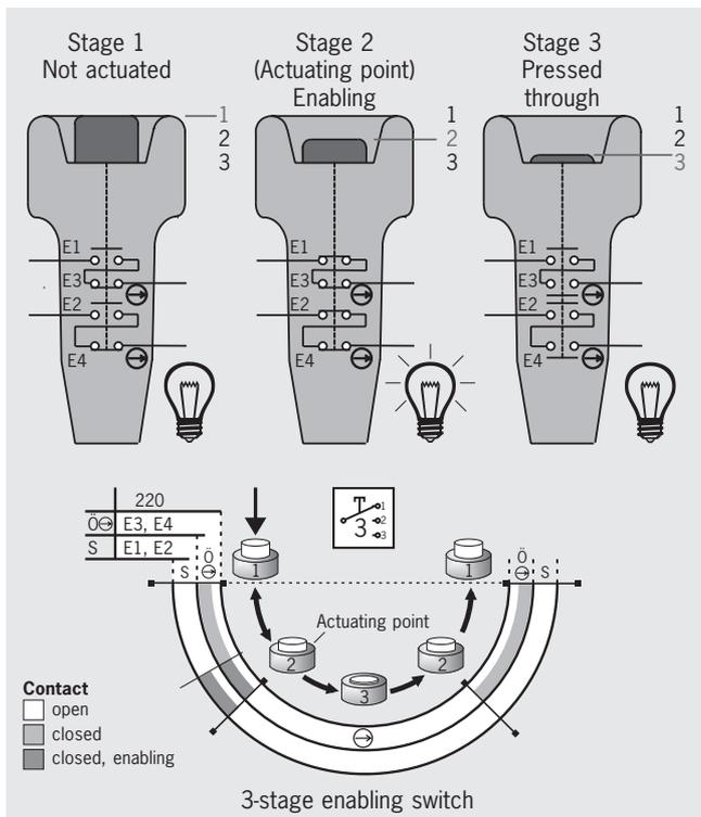
As can be clearly seen in the figure, the enabling function can only be achieved at stage 2. This function is provided by the closing of the normally open contacts (NO = E1 and E2). If the button is released, that is back from stage 2 to stage 1, the normally open contacts are opened again. The 2 and 3-stage enabling switches are identical in this function.
