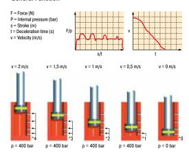
\* The load velocity reduces continuously as you travel through the stroke due to the reduction in the number of metering orifices (\*) in action. The internal pressure remains essentially constant and thus the Force vs. stroke curve remains linear
