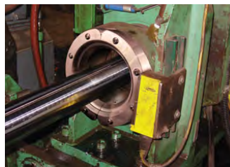
A Model 2404 4" (102mm) Super Air Wipe cleans a steel rod after processing.
