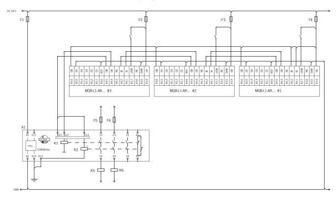
Important: In accordance with the risk analysis, the application must be evaluated using a feedback loop (not shown here).
