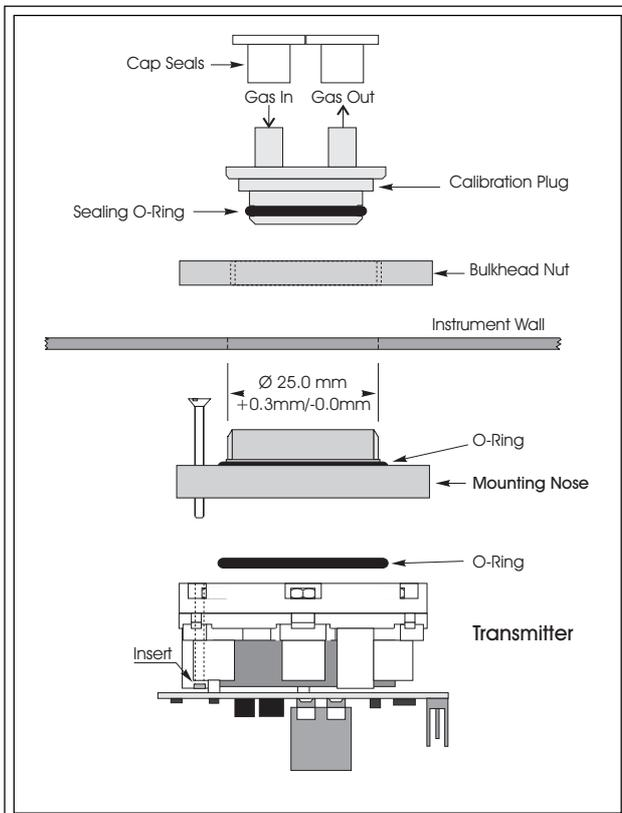
The Mounting Nose also features a plug for easy zeroing and exposure to gas during calibration. A bonded membrane and mesh is included to prevent the ingress of dirt and dust particles to the CiTiceL.
