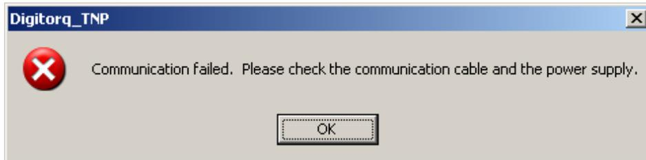
The above error will appear if the TNP Digital Torque meter is OFF or the COM port selected from the list is not correct.
