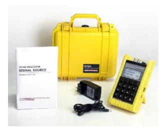
The <u>1510A Precision Signal Source generator</u> available from MTI Instruments is a compact and portable device and includes dual-channel Direct Digital Synthesis (DDS) that creates high precision signals over a wide frequency and amplitude range.
