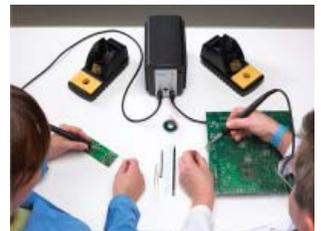
A third option for the system is the MFR-H4-TW Precision Tweezers Hand-piece. This hand-piece is ideal for SMD removal of 0201 resistors to 28 mm long SOIC.
