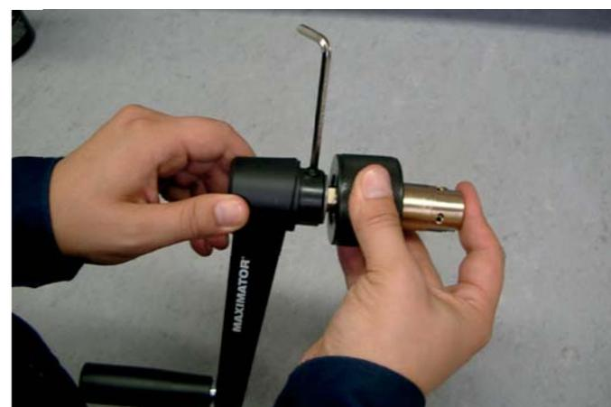
Use the supplied hexagonal offset screwdriver to loosen the headless set screw that keeps the crank handle in its position.
