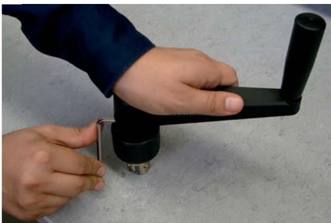
Align the crank handle and blanking die holder in such a manner that the head-less set screw of the crank handle pushes onto the key area at the shaft of the blanking die holder.
