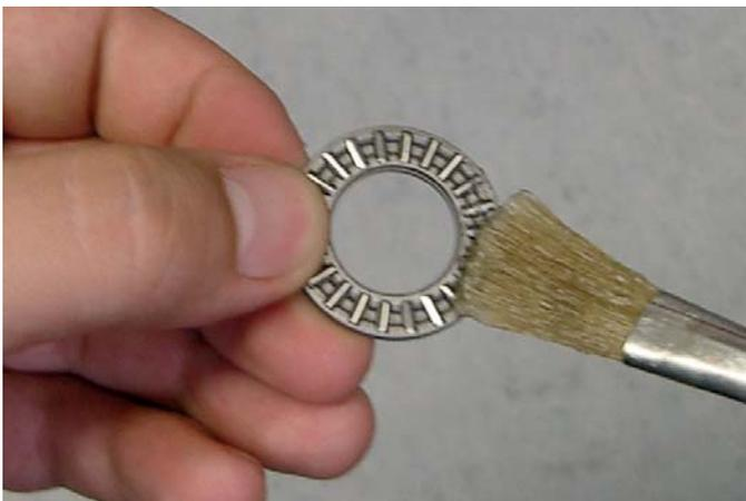
Lubricate the needle bearings with roller bearing grease.
