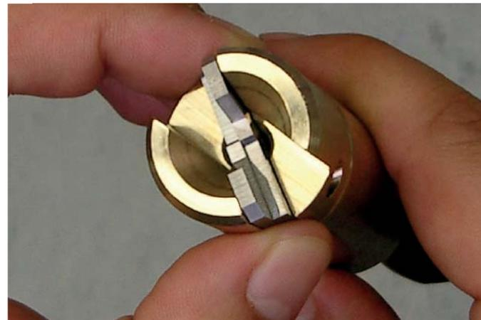
Insert the blanking dies into the blanking die holder as shown in the illustration. Make sure that the labelled order code is always on the outside.
