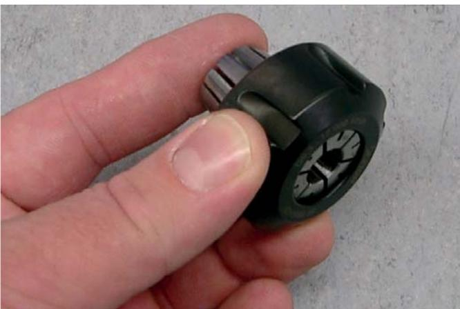
Push the collet chuck into the tensioning nut.
