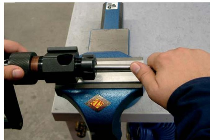
Insert the pipe into the collet chuck. Push forward till to the cheek and pull backward for approx.1 mm
