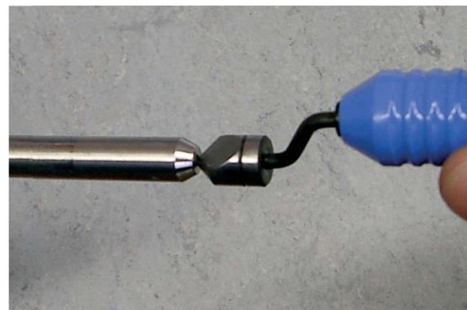
The only work left to do now is debur-ring of the internal diameter of the finished pipe. Carefully remove all chips that are generated by taper cutting edges and deburring (inside and out-side).
