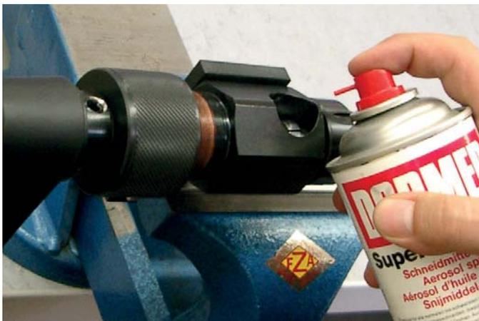
Apply cutting oil onto the blanking dies and pipe end through the side opening in the base structure. Repeat several times during the cutting operation.
