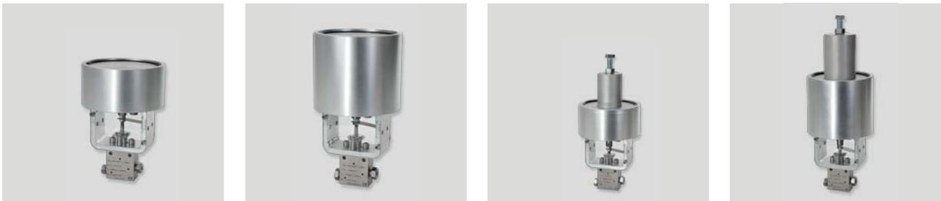
MAXIMATOR air operated valve actuators are piston type design, and are mounted on a manual valve to provide remote control capability. There are two air to open actuators and two air to close actuators available, and selection is based on the valve size, system pressure, and air pressure available.
