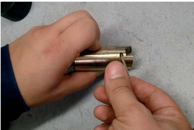
Loosen the 4 headless set screws in the blanking die holder to disassemble the blanking dies. Then remove the blanking from the blanking die holder.
