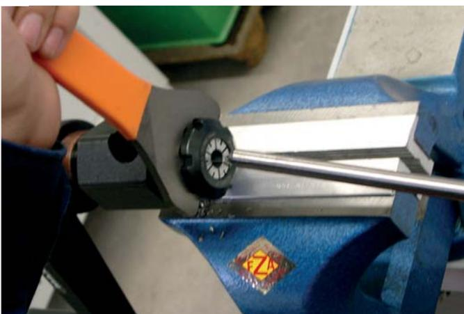
Use the chuck key to loosen the tensioning nut and the tube can be re-moved from the coning tool.
