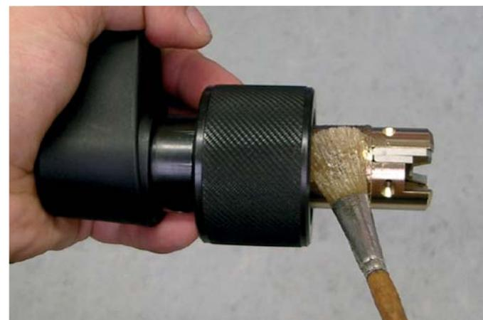
Lubricate the running surface of the blanking die holder.
