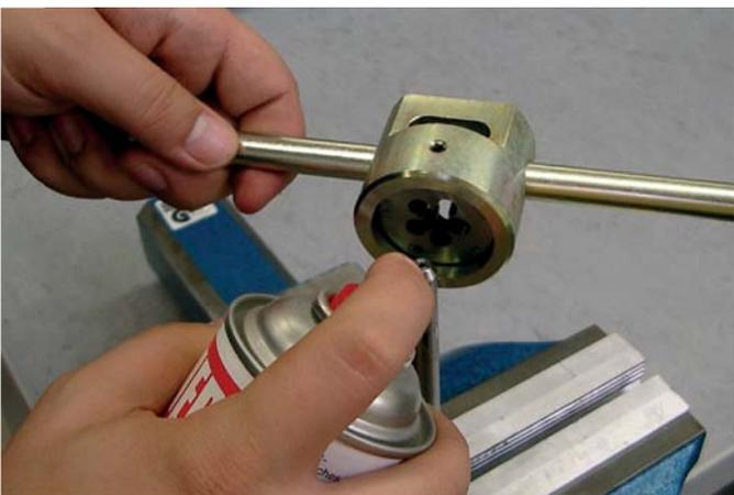
Wet the pipe and the die with cutting oil.
