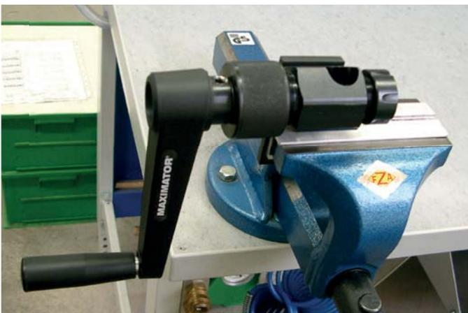
Clamp the coning tool on the fixing plate in a vice or similar.
