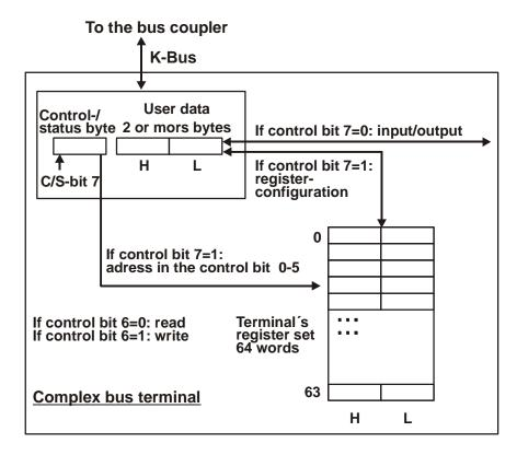
The control or status byte occupies the lowest address of a logical channel. The corresponding register values are located in the following 2 data bytes. (The BK2000 is an exception: here, an unused data byte is inserted after the control or status byte, and the register value is therefore placed on a word boundary).
