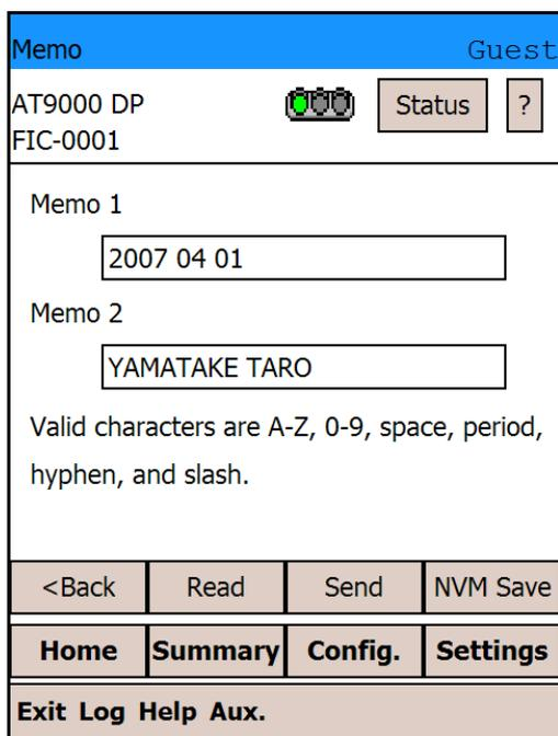
Memo creation is now complete. If you might need to turn off the power of the device within 30 seconds after the transmission of the data, tap [NVM Save] to save your changes. Tapping [Read] reads the set values and displays them again. Tapping [<Back] restores the original screen.
