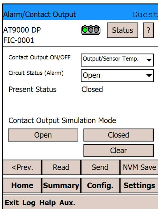
If you might need to turn off the power of the device within 30 seconds after the transmission of the data, tap [NVM Save] to save your changes.
