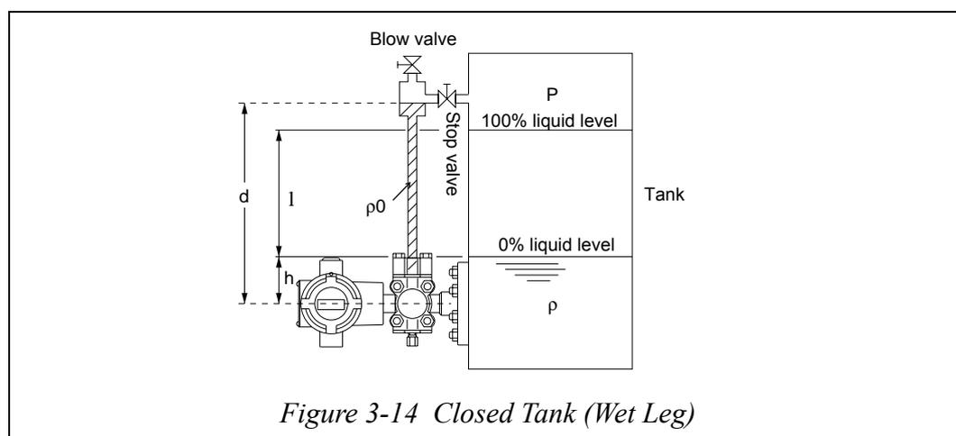
Differential pressure at 0% liquid level (Pressure on high-pressure side - Pressure on low-pressure side) =  $d\rho_0 - h\rho = \text{LRV}$
