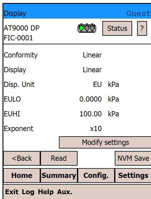
Indicator configuration is now complete. If you might need to turn off the power of the device within 30 seconds after the transmission of the data, tap [NVM Save] to save your changes. Tapping [Read] reads the set values and displays them again. Tapping [<Back] restores the original screen.
