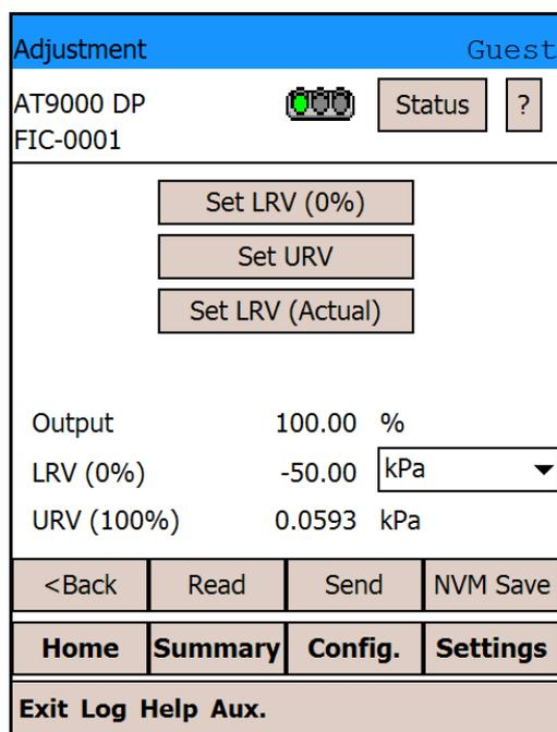
(5) URV adjustment is now complete. If you might need to turn off the power of the device within 30 seconds after the transmission of the data, tap [NVM Save] to save your change. Tapping [Read] reads the set values and displays them again. Tapping [<Back] restores the original screen.
