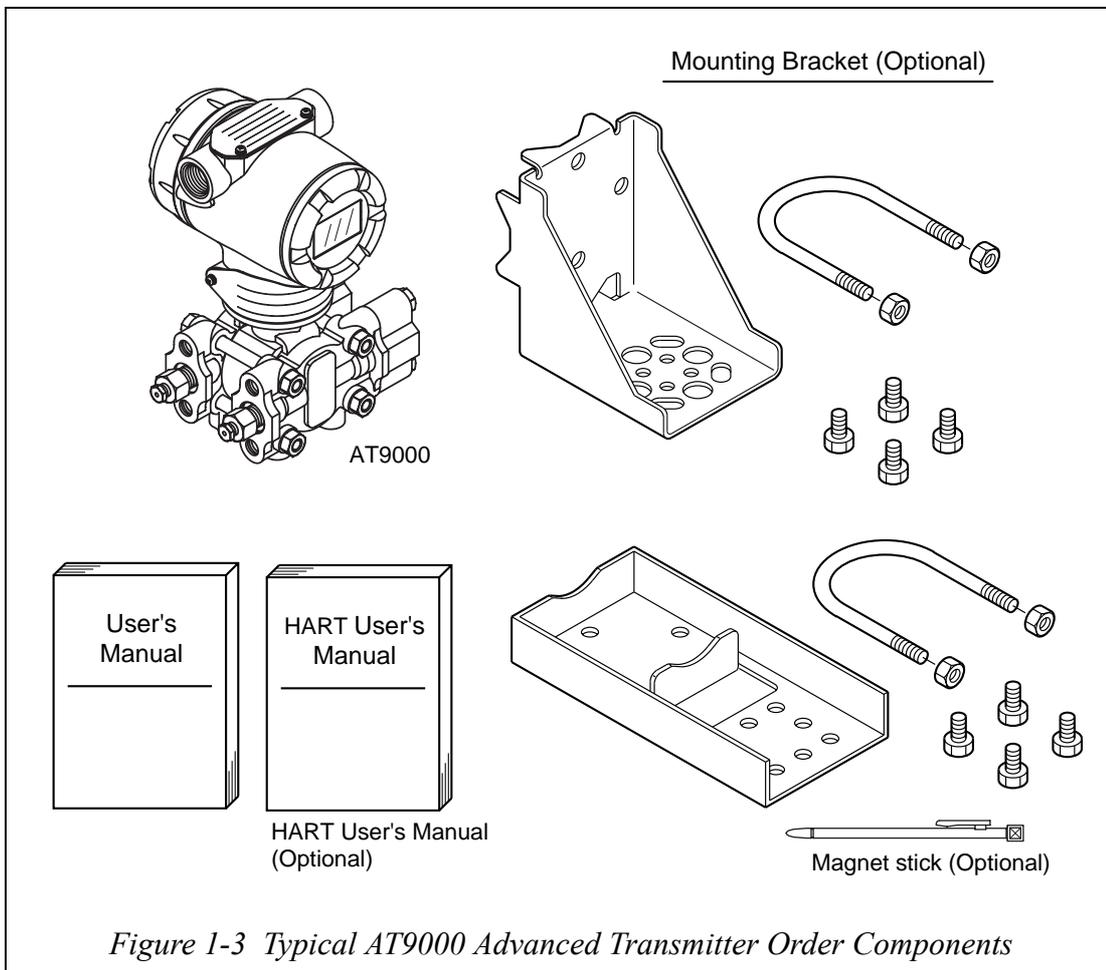
Figure 1-3 Typical AT9000 Advanced Transmitter Order Components
