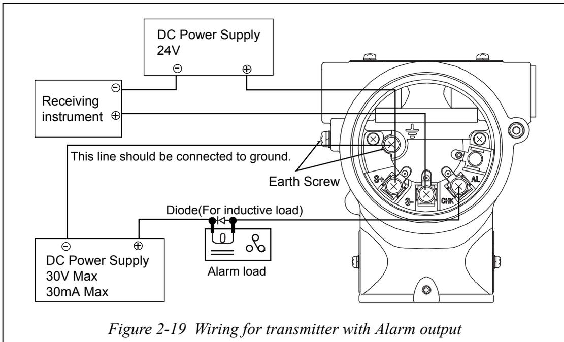
**~Note** *Current cannot checked for a transmitter with alarm contact output.*
