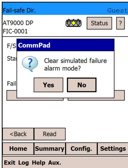
The Burnout Simulation is now cleared. Note that even if you do not clear the Burnout Simulation, the device will automatically clear it after approximately 10 minutes without communication.
