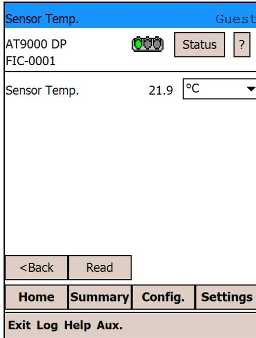
Tapping [Read] reads the sensor temperature and displays them again. Tapping [<Back] restores the original screen.
