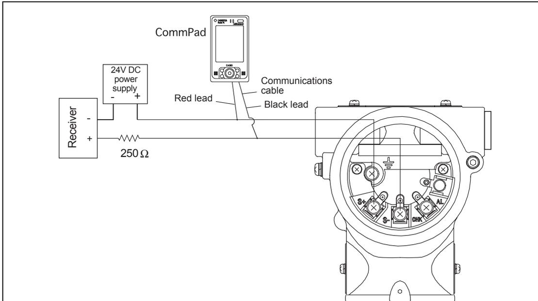
Note: Always connect CommPad's communications cable to the loop wiring as follows:
