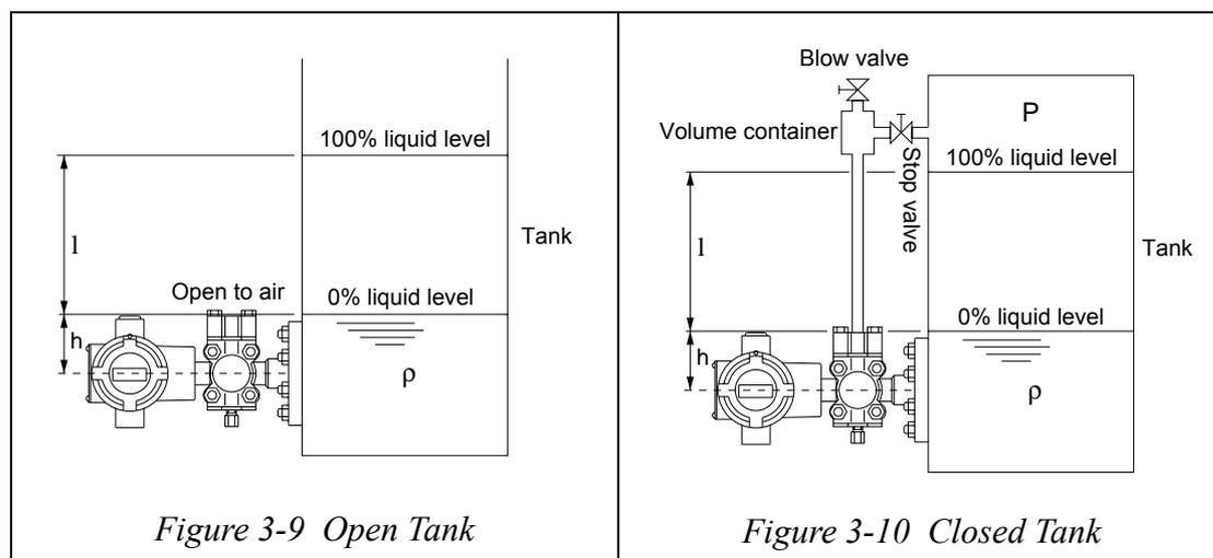
Differential pressure at 0% liquid level (Pressure on high-pressure side - Pressure on low-pressure side) =  $h\rho = \text{LRV}$
