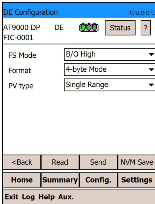
If you might need to turn off the power of the transmitter within 30 seconds after the transmission of the data, tap [NVM Save] to save your change.
