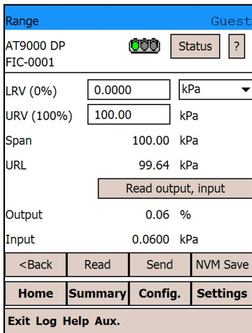
(9) Tapping [Read output, input] reads the output and input value and updates the displays. If you might need to turn off the power of the device within 30 seconds after the device of the data, tap [NVM Save] to save your changes.
