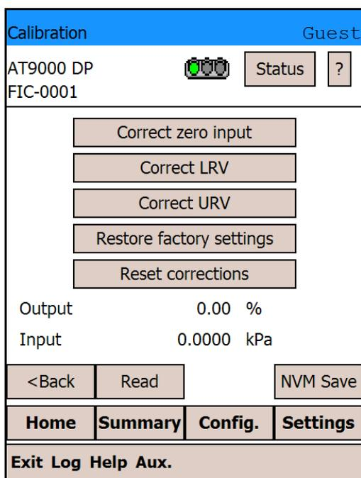
(5) Correct zero input is now complete. If you might need to turn off the power of the device within 30 seconds after the transmission of the data, tap [NVM Save] to save your change. Tapping [Read] reads the set values and displays them again. Tapping [<Back] restores the original screen.
