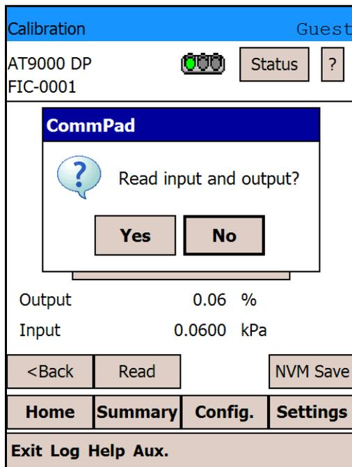
(4) Input has now changed approximately to zero as a result of the calibration.
