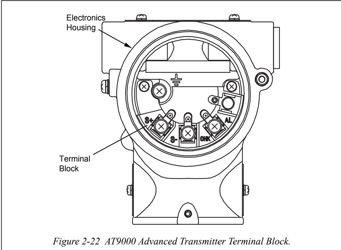
*Figure 2-22 AT9000 Advanced Transmitter Terminal Block.*
