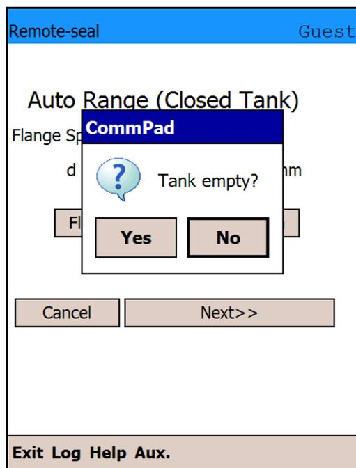
The approximate distance between the flanges will be calculated based on the current input values and the density of the fill fluid. If the value is acceptable, tap [Next>>].
