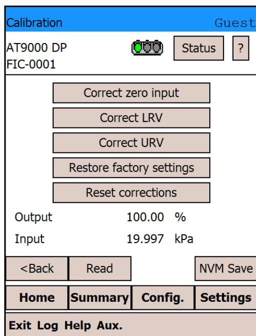
(5) Correct URV is now complete. If you might need to turn off the power of the device within 30 seconds after the transmission of the data, tap [NVM Save] to save your change. Tapping [Read] reads the set values and displays them again. Tapping [<Back] restores the original screen.
