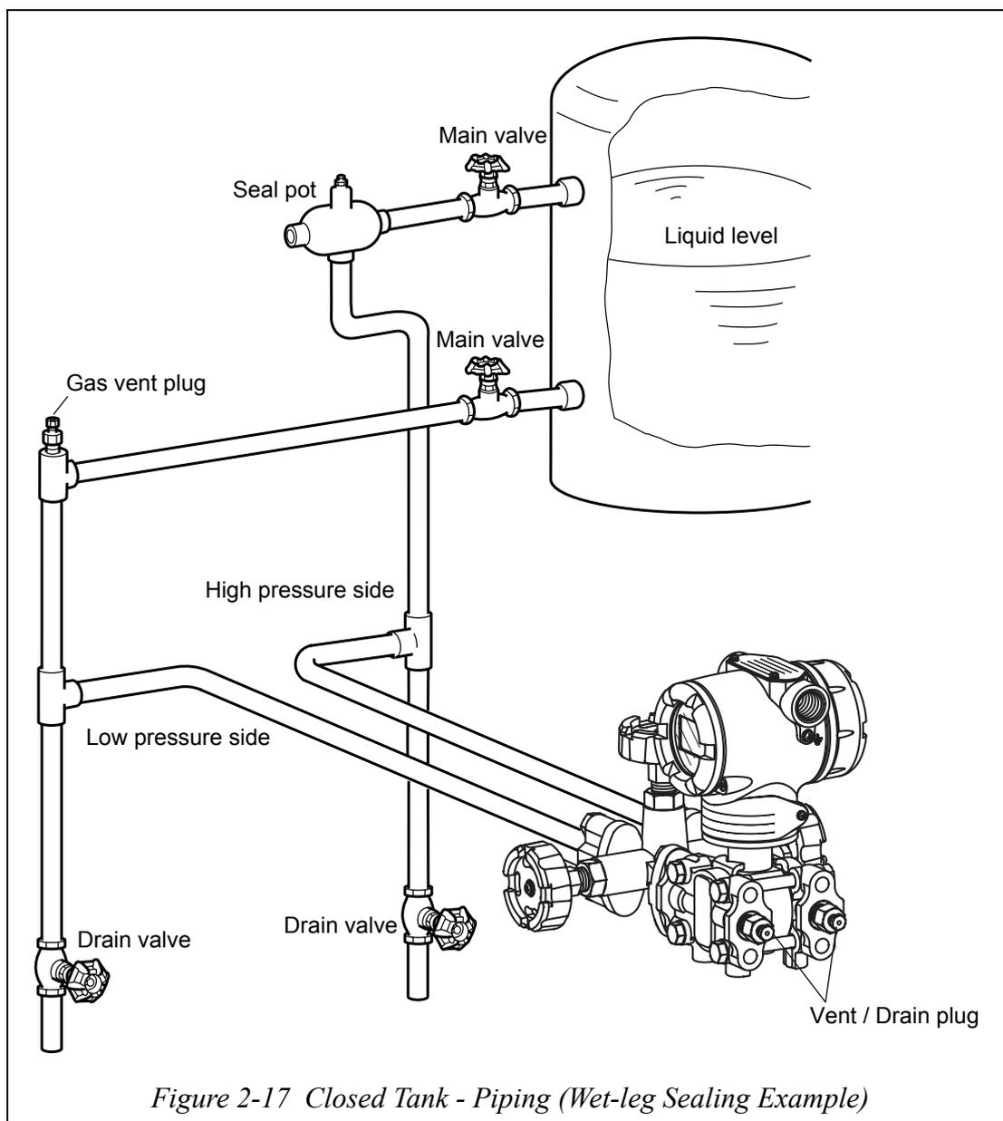
*Figure 2-17 Closed Tank - Piping (Wet-leg Sealing Example)*
