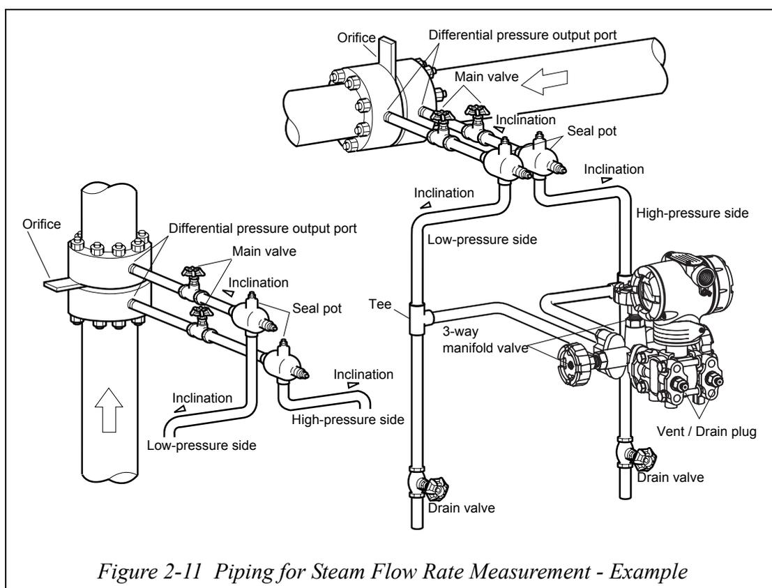
Figure 2-11 Piping for Steam Flow Rate Measurement - Example
