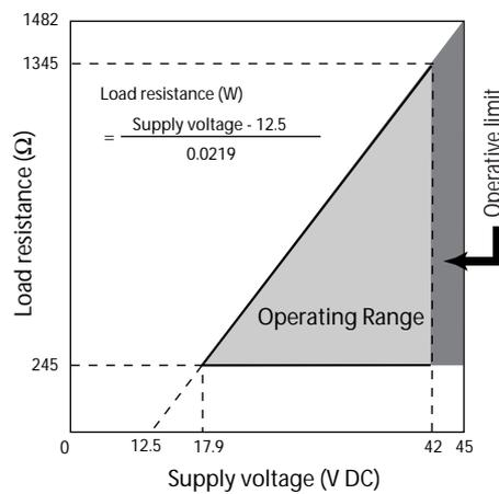
Figure A-2 Supply voltage vs. load resistance
