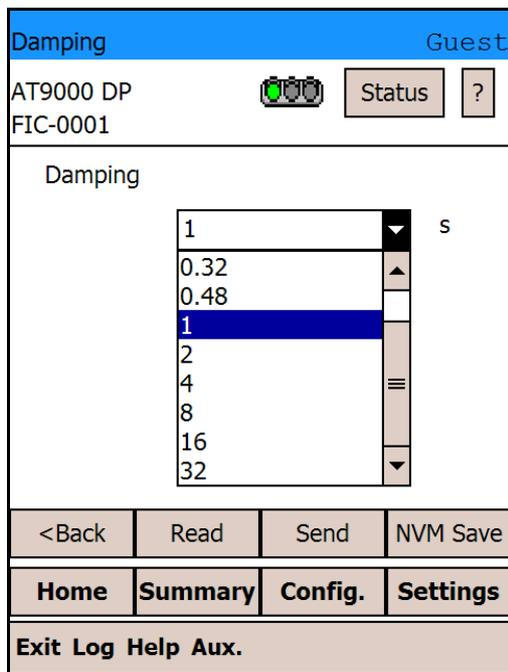
Damping time configuration is now complete. If you might need to turn off the power of the device within 30 seconds after the transmission of the data, tap [NVM Save] to save your change. Tapping [Read] reads the set values and displays them again. Tapping [<Back] restores the original screen.
