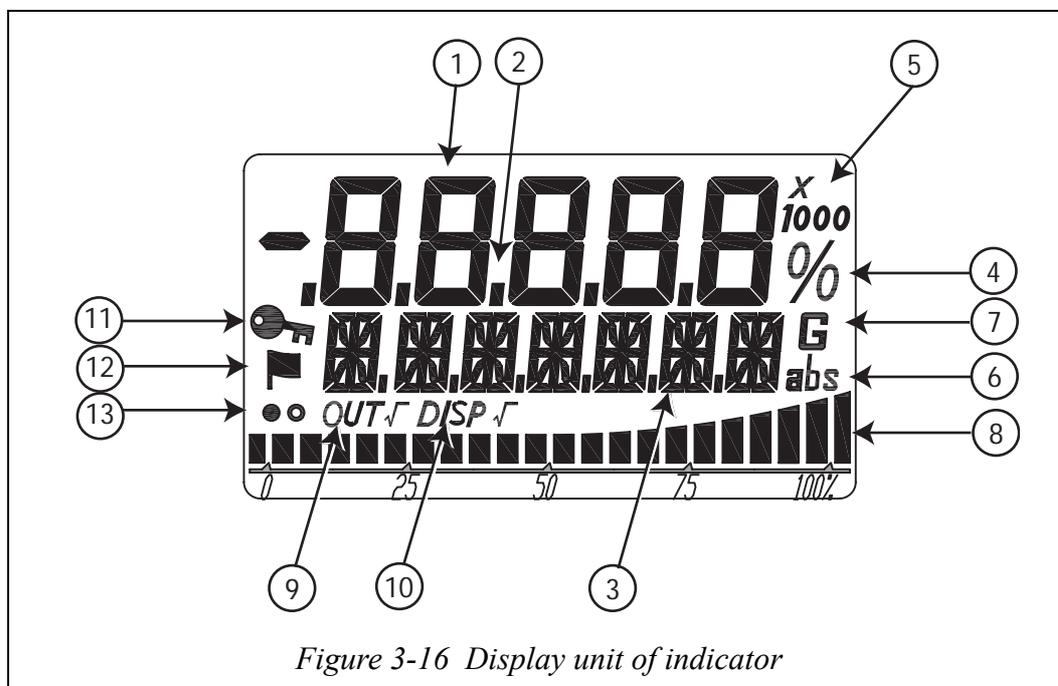
Figure 3-16 Display unit of indicator
