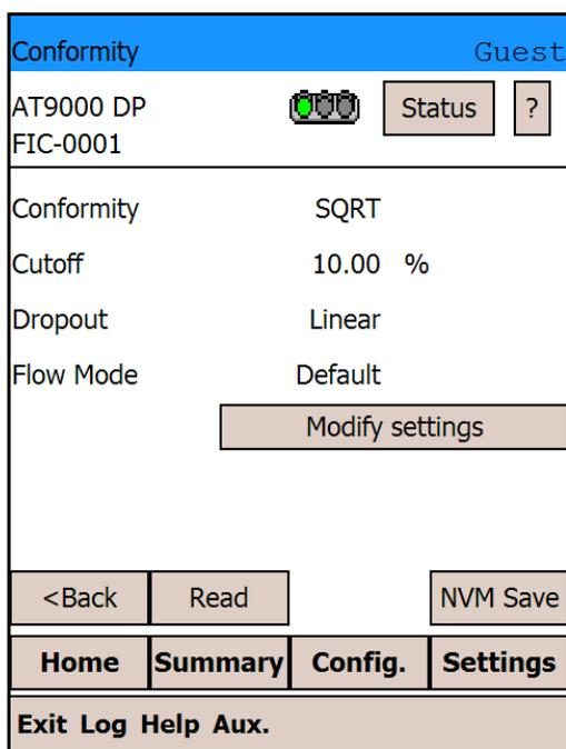
The configurations for conformity are now complete. If you might need to turn off the power of the device within 30 seconds after the transmission of the data, tap [NVM Save] to save your changes. Tapping [Read] reads the set values and displays them again. Tapping [<Back] restores the original screen.
