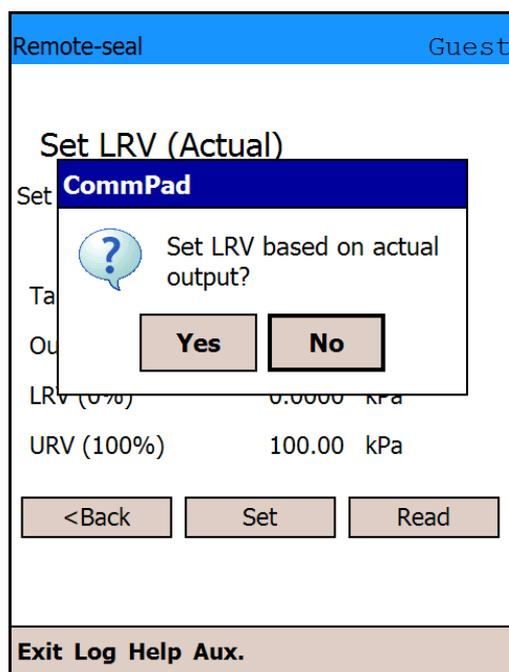
The range changes, and the Output value becomes identical to that of Target.
