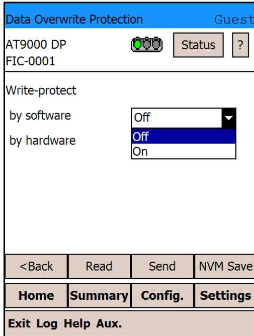
If you might need to turn off the power of the device within 30 seconds after the transmission of the data, tap [NVM Save] to save your change. Tapping [Read] reads the set values and displays them again. Tapping [<Back] restores the original screen.
