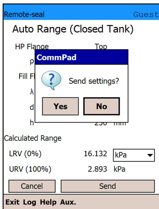
(14) The remote-seal auto range process is now complete. If you might need to turn off the power of the transmitter within 30 seconds after the transmission of the data, tap [NVM Save] to save your changes.
