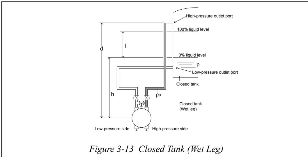
Figure 3-13 Closed Tank (Wet Leg)
