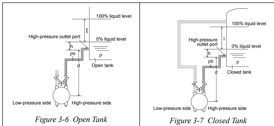
Differential pressure at 0% liquid level (Pressure on high-pressure side - Pressure on low-pressure side) =  $h\rho + d\rho_0 = \text{LRV}$
