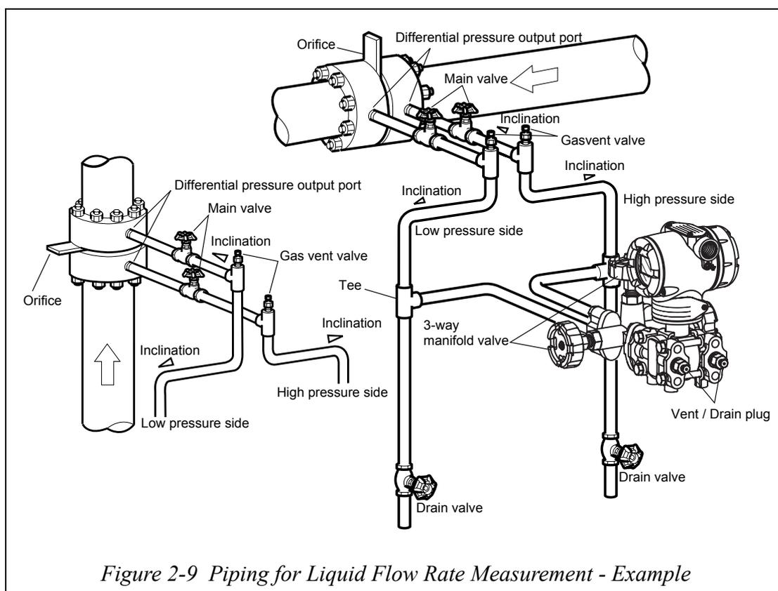
This transmitter is located underneath the differential pressure output port of the process pipe.
