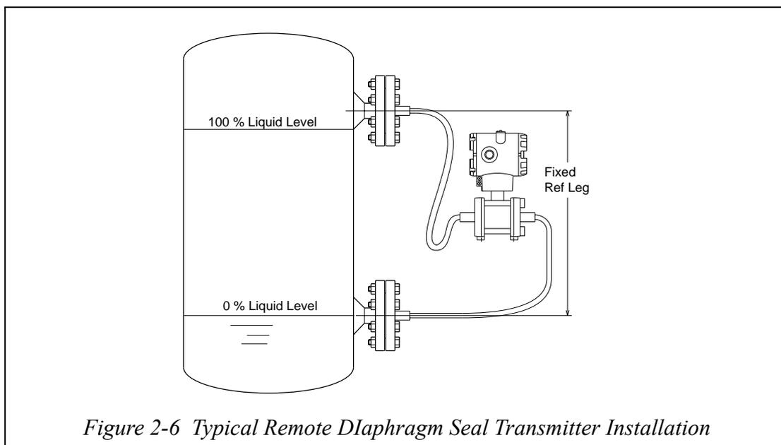
Figure 2-6 Typical Remote Diaphragm Seal Transmitter Installation
