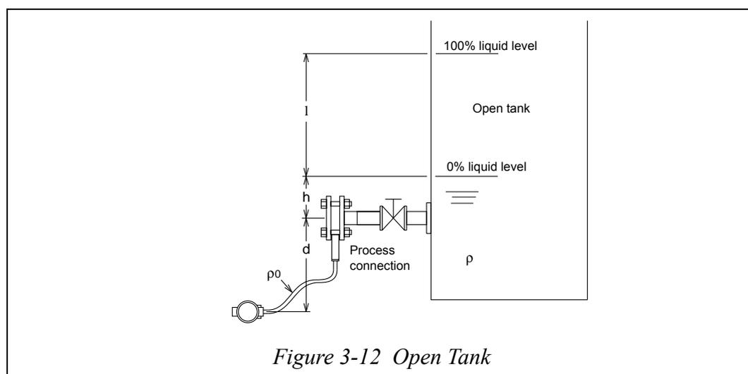
Differential pressure at 0% liquid level =  $h\rho + d\rho_0 = \text{LRV}$
