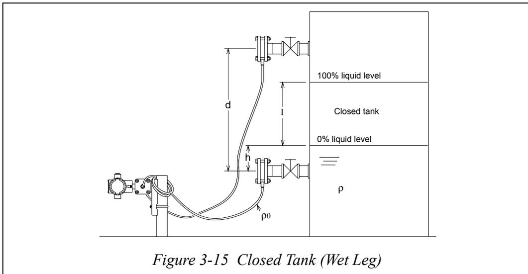
Figure 3-15 Closed Tank (Wet Leg)
