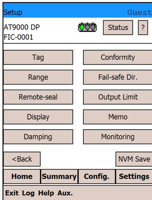
Nonfunctional buttons on the screen are displayed in gray. The following buttons are nonfunctional under the specified conditions:
