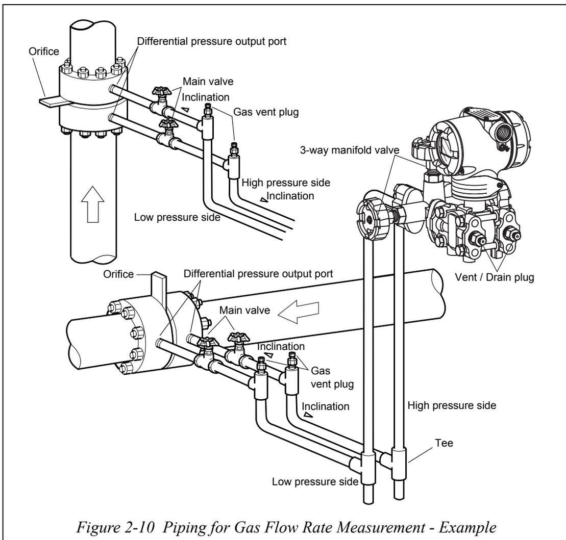
*Figure 2-10 Piping for Gas Flow Rate Measurement - Example*
