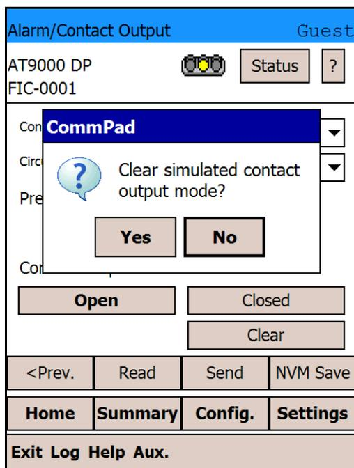
The Contact Output Simulation Mode is now cleared. Note that even if you do not clear the Contact Output Simulation Mode, the device will automatically clear it after approximately 10 minutes without communication.
