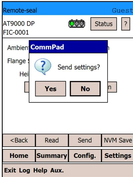
(8) The ambient temperature compensation configuration is now complete. If you might need to turn off the power of the transmitter within 30 seconds after the transmission of the data, tap [NVM Save] to save your changes.
