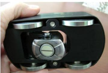
The **EZ Scan 4** is a small, single axis linear B-Scan encoder, for use with the T-Gage V DLC, with magnetic wheels and a couplant delivery system. Ideal applications include storage tank bottom and side walls, flat plates and pipes with a 10 cm (4") or greater outside diameter. The scanner comes as standard with a 5Mhz dual transducer spring loaded in two directions, other transducers are also available.
