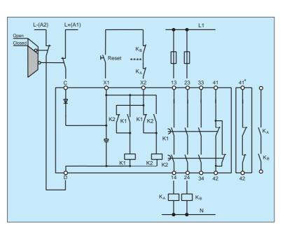
Example for dual-channel door monitoring using two limit switches (one with positive opening contacts) and external reset button.
