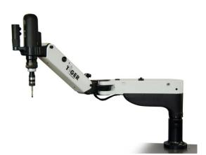
The machine itself consists of a radial arm joint to a tilting arm balanced by means of a pneumatic spring. The head member and the electric motor find themselves at the end of the tilting arm and is adapt to always move at right angle with respect to its working area.
