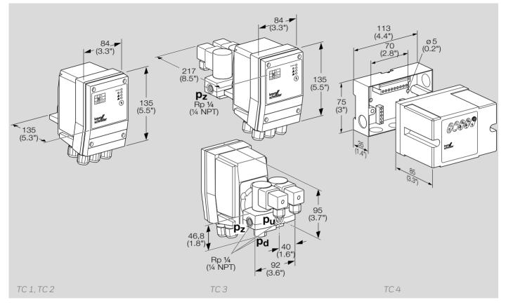
Inlet pressure connection =  $p_u$ , intermediate pressure connection =  $p_z$  and the outlet pressure connection =  $p_d$
