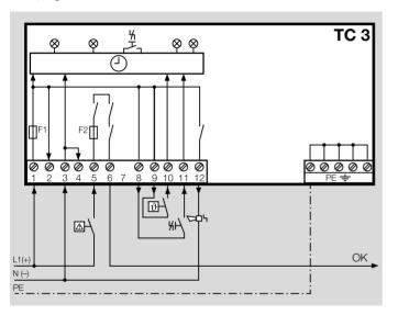
Remote reset by applying control voltage to terminal 11 or via a floating contact between terminals 8 and 11.
