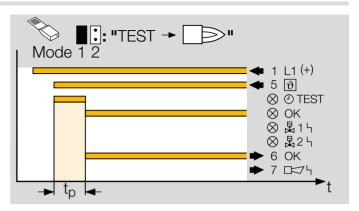
If the tightness control TC detects a leak on one of the two valves, the red LED lights up for a fault on valve V1 1 or valve V2 2 A fault is signalled externally 2, e.g. by switching on a buzzer or a warning light.
