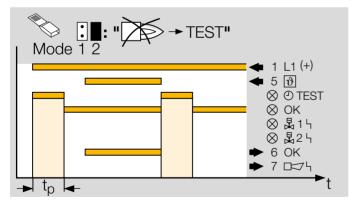
If the tightness control TC detects a leak on one of the two valves, the red LED lights up for a fault on valve V1 1 or valve V2 2 2 A fault is signalled externally 2 A, e.g. by switching on a buzzer or a warning light.
