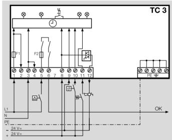
Remote reset by applying control voltage (+24 V) to terminal 11.
