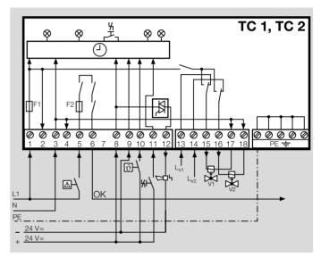
V1 = inlet valve, V2 = outlet valve.
