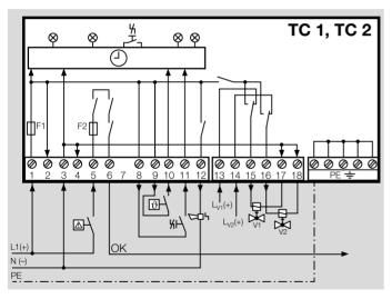
V1 = inlet valve, V2 = outlet valve.
