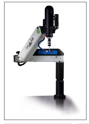
The machine is formed by a tilting arm being by means of a pneumatic spring, said arm being fitted through an intermediary union to a radial arm being revolvable around 360°. The assembly is secured to the workbench by means of a base plate being provided with a post clearing the whole table area.
