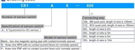
① Note: The quick joint that is attached at the end of wire is three-needle-male joint-linear-rotary screw thread type. The female joint plug has to be ordered additionally. Please refer to PVI-49 for the specific data.
