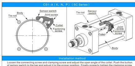
of sensor switch to the bar and adjust it to the proper position. Finally properly tighten the clamping screw
