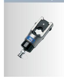
Hydraulic crimper head with removable die-holder, complete with male Quickfit automatic coupler for connection to hydraulic pump units with a working pressure of 700 har
