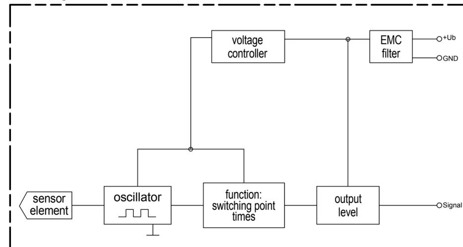
**Functional diagram for MINIMUM Probes <sup>ⓑ</sup>**
