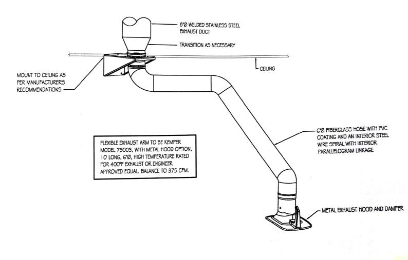
FLEXIBLE EXHAUST ARM DETAIL SCALE: NONE
