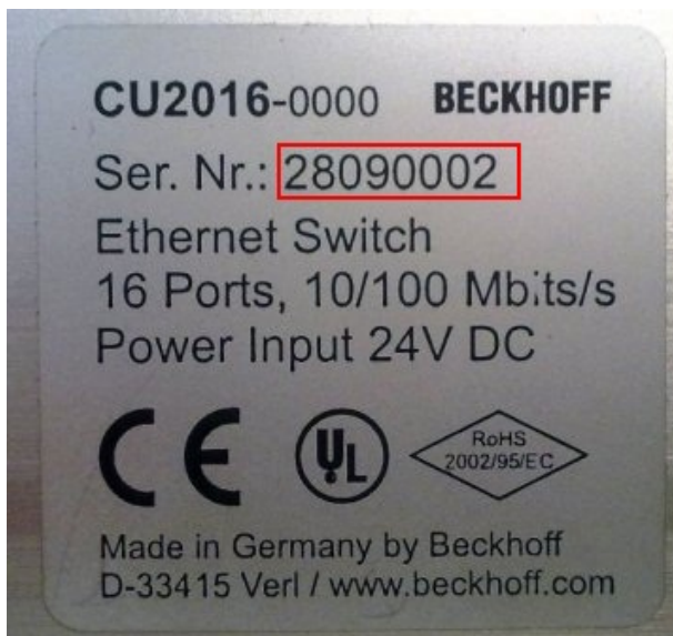
Fig. 3: CU2016 switch with batch number
