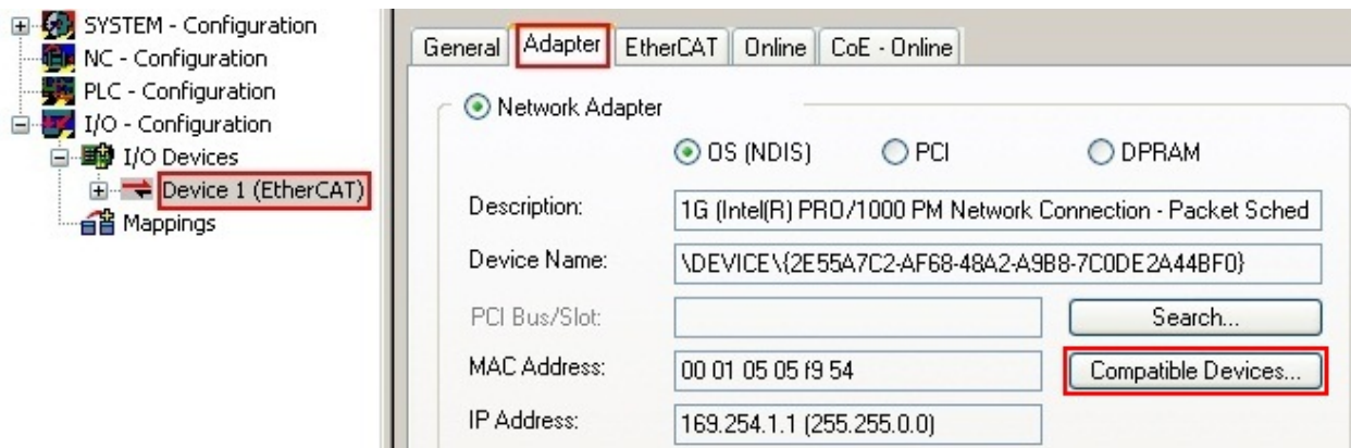
Fig. 88: EtherCAT device properties(TwinCAT 2): click on „Compatible Devices...“ of tab “Adapter”
