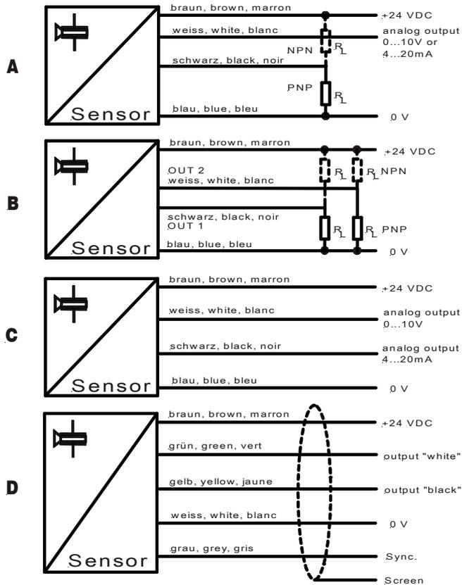
All versions with integrated cable instead of connector have cable colours according to scheme "D".
