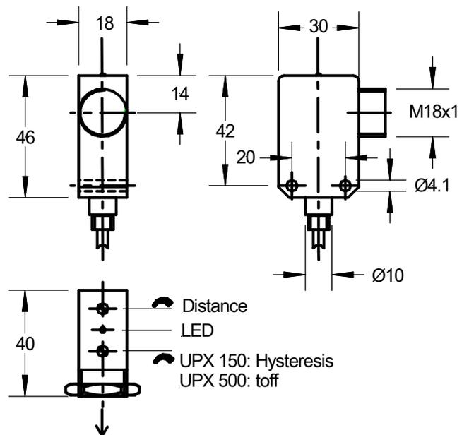
Use the miniature screw driver which is included for adjustment of the two potentiometers.
