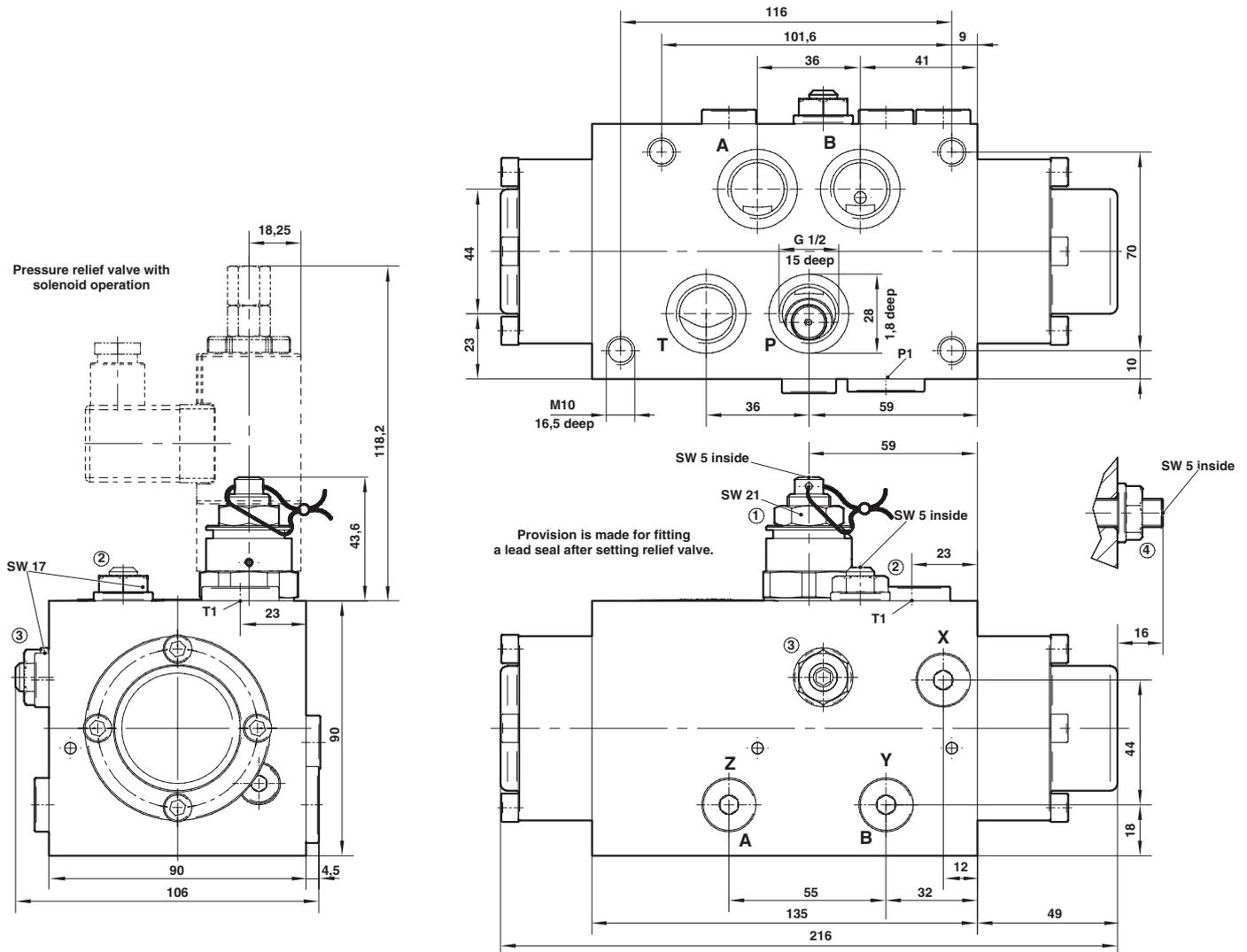
For subplate mounting 4 O-Rings 23.47 x 2.62 (PRP-No. 119) are necessary. They are not included with valves without subplates (Part-No. 12 425 56).
