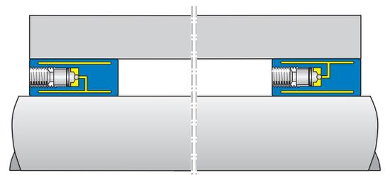
*This ETP-AXPRESS is used for fastening and centering of a cylinder in a printing machine for beverage cans of aluminium. It has two separate pressure chambers, one for expansion to the shaft and one to the bore of the cylinder. The runout is better and downtime much shorter than with the mechanical clamping used before*
