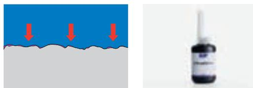
**ETP-FRICTION** is a liquid containing extremely small, hard, irregular particles which "grips into" the contact surfaces. It is easily applied with a brush or cloth. ETP-FRICTION will not harden or cure. Content in the can: 125 ml.
