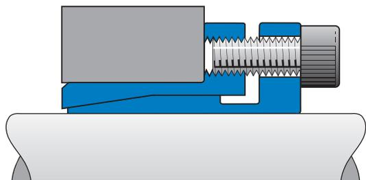
*The inner sleeve of ETP-MINI has a light recess close to the flange in order to create a more uniform surface pressure to the shaft.*
