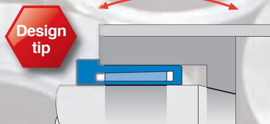
Long thin rollers subjected to high bending torque, can be fastened to stub shafts with ETP-HYLOC. To decrease the elastic deformation of the roller and make it easier to take up the bending torque, the inner part of the hub and the stub shaft can be designed with conical support surfaces. ETP-HYLOC gives good concentricity and fast changes.
