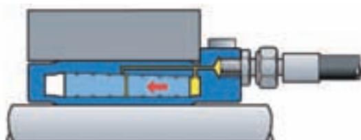
*Dismantling: apply pressure in the "OFF" and "P" (not shown) connections. ETP-HYLOC returns to its original measurements and the joint is loose.*
