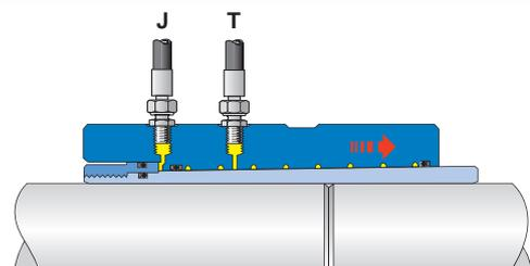
**Mounting:** with an oil pump the outer sleeve is driven up onto the inner sleeve. When mounted there is no hydraulic pressure. The small conical angle prevents the outer sleeve from releasing.
