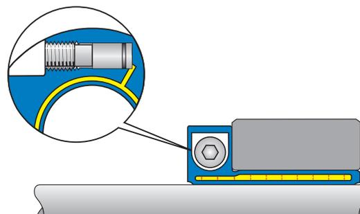
*When the pressure screw is tightened to the recommended tightening torque, the piston has reached the bottom of the bore. ETP-EXPRESS R has created a uniform surface pressure against the shaft and hub.*
