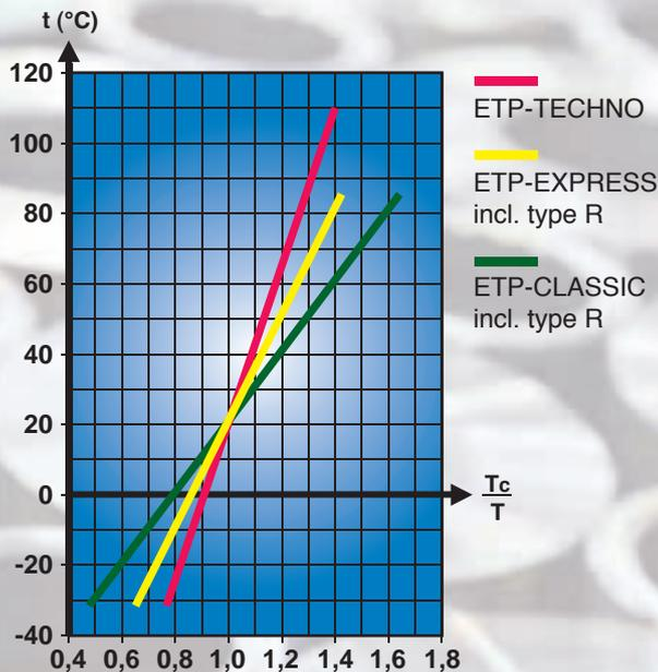
The pressure medium in hydraulic ETP connections and the double-walled steel sleeve have different volume expansion coefficients. This means that when the temperature rises, the pressure in the connection increases and a higher torque can be transmitted. The opposite is valid at decreasing temperature. Also the seals built into the connections decides the upper and lower operating temperatures.
