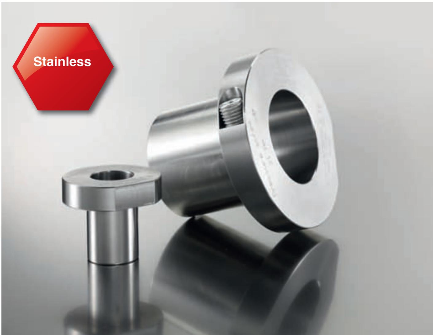
ETP-EXPRESS R is available as standard for shafts 15-80 mm, also imperial. Runout  $\leq 0,02$  mm. Number of mountings 200 – 800 (size dependent). The extremely thin built-in dimensions allows for a compact design with low weight and inertia.
