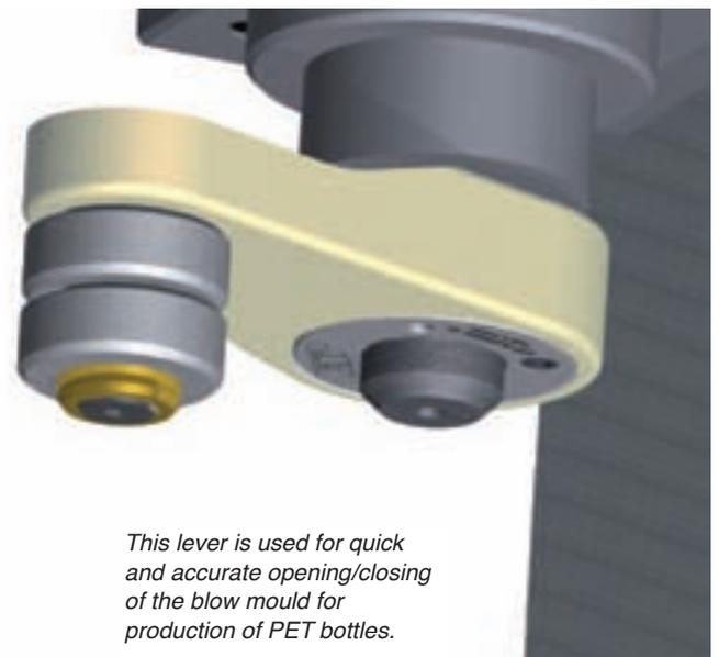
*This lever is used for quick and accurate opening/closing of the blow mould for production of PET bottles.*
