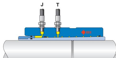
**Dismantling:** the outer sleeve is in a controlled way driven back to its origin. The inner sleeve releases the contact to the shaft and the joint can be dismantled.
