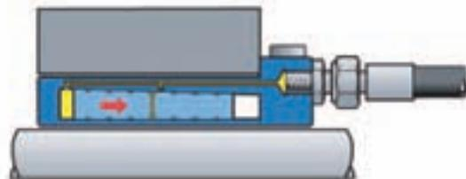
*Mounting: apply pressure in the "ON" and "P" (not shown) connections. When mounted no hydraulic pressure remains. The small conical angle prevents the piston from releasing.*
