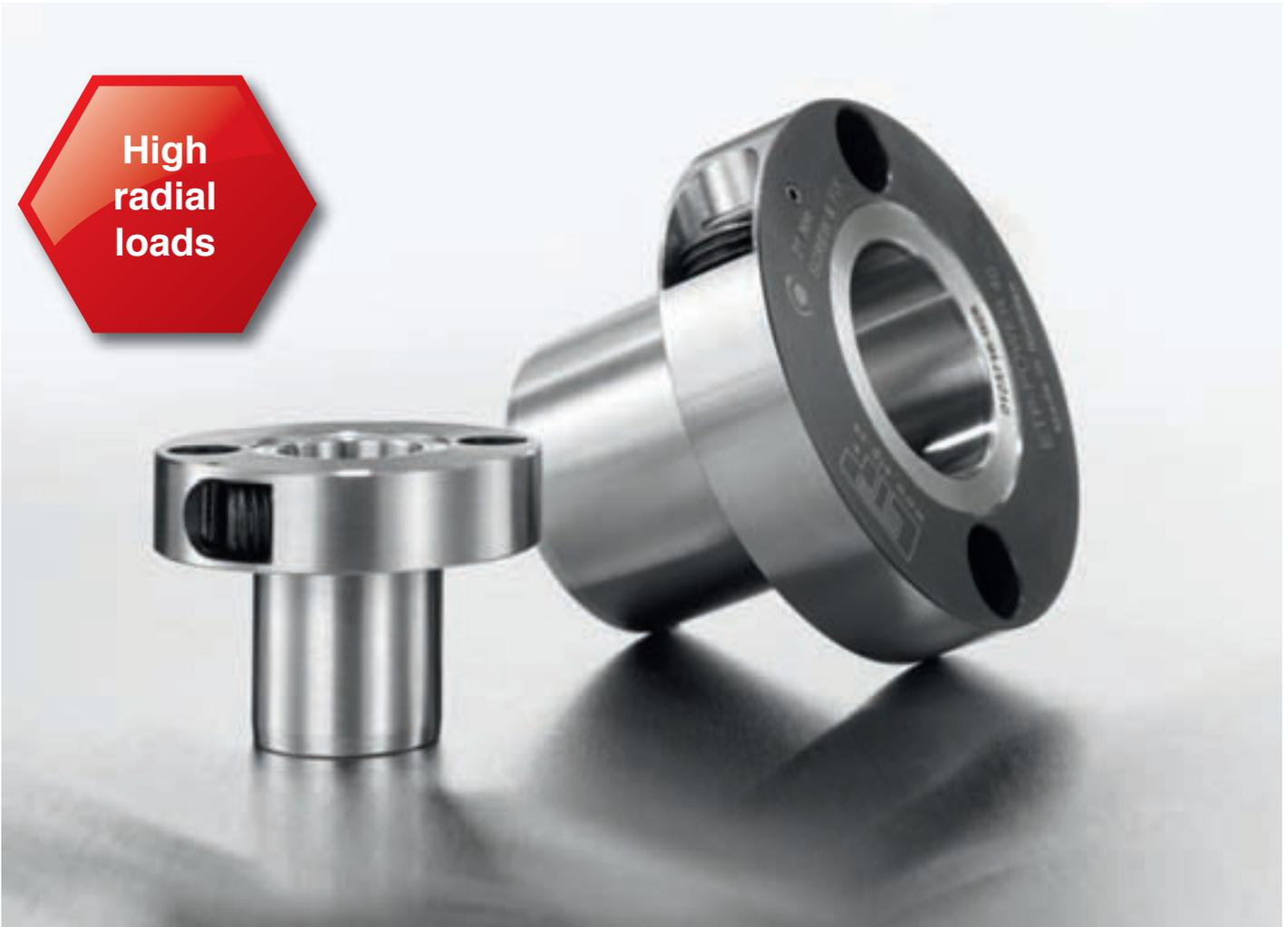
ETP-POWER is available as standard for shafts 15 – 40 mm. Runout  $\leq 0,03$  mm. Number of mountings 200 - 500 (size dependent). ETP-POWER combines quick mounting with a high radial load capacity due to the specially developed pressure medium.
