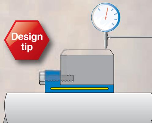
When manufacturing precision gears, they can be fastened with ETP- EXPRESS. If the gear is fixed in its position with an axial screw or pin before the last grinding operation, a repeatability within 2  $\mu\text{m}$  will be achieved.
