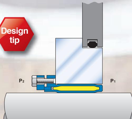
At varying temperature and with a hub made from aluminium ETP-connections can be used. Because of the even surface pressure and the lack of slotted sleeves, ETP-connections can function as a sealing element up to a pressure difference,  $p_1 - p_2$ , of 50 bar.
