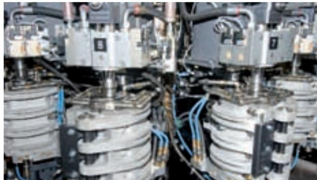
*Complete blow mould unit with several moulds/cavities.*
