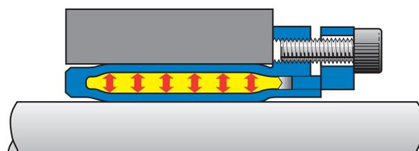
When the screws have been tightened, ETP-CLASSIC creates an even surface pressure against the hub and shaft along virtually the entire length.
