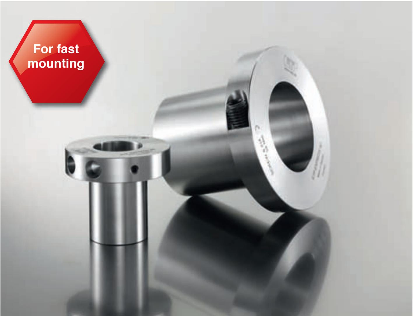
ETP-EXPRESS is available as standard for shafts 15-100 mm, also imperial. Runout  $\leq 0,02$  mm. Number of mountings 500 - 2 000 (size dependent). The extremely thin built-in dimensions allows for a compact design with low weight and inertia.
