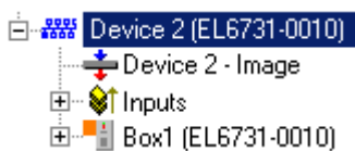
Fig. 124: Adding a „Profibus Slave EL6731, EtherCAT“ in the TwinCAT tree
