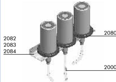
Mounting support with protective cover for simalube
