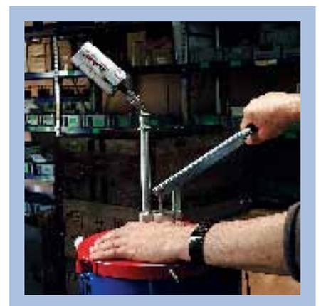
simalube can be filled as well as refilled by using a standard barrel pump that is typically used to fill grease guns.
