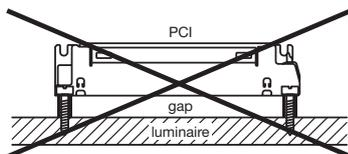
If several ballasts are installed in masts, boxes, etc., measures must be taken to avoid overheating of individual components.
