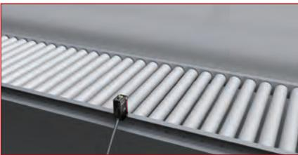
At the factory default setting, the sensor is constantly triggered by background.
