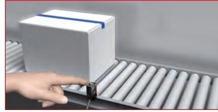
Sensor is adjusted to appropriate sensitivity.
